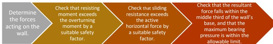
**Fig. 2.** The procedure of stability analysis.
