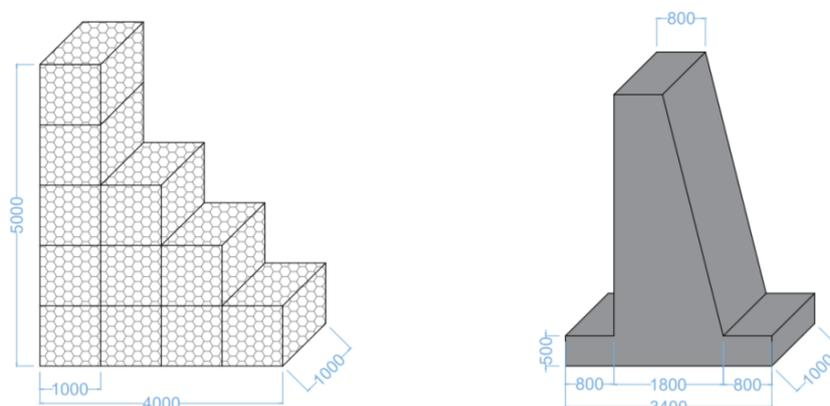
**Fig. 4.** The optimize layout and dimension of retaining wall
