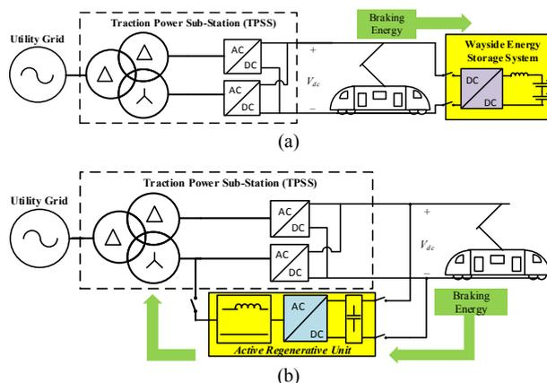
Fig. 1: Regenerative braking energy recovering solutions in railway traction (a) Wayside Energy Storage System (WESS), (b) Active Regenerative Unit [9].
