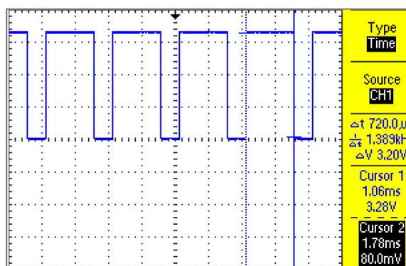
Fig. 5. Execution time of the RMS computation for written C code
