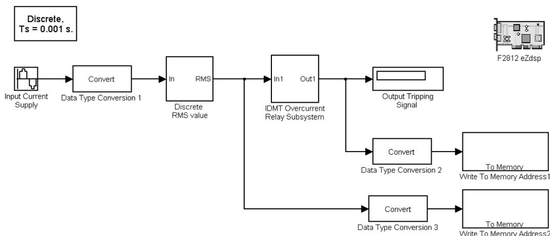
Fig. 1. The simulation model of overcurrent relay
