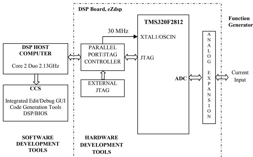
Fig. 4. The block diagram of the basic configuration for eZdsp TMS320F2812
