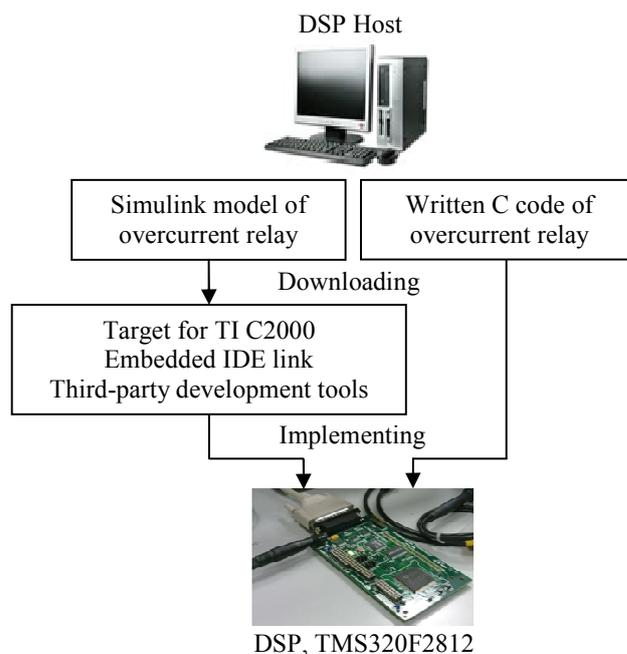
Fig. 3. Hardware implementation of overcurrent relay on TMS320F2812
