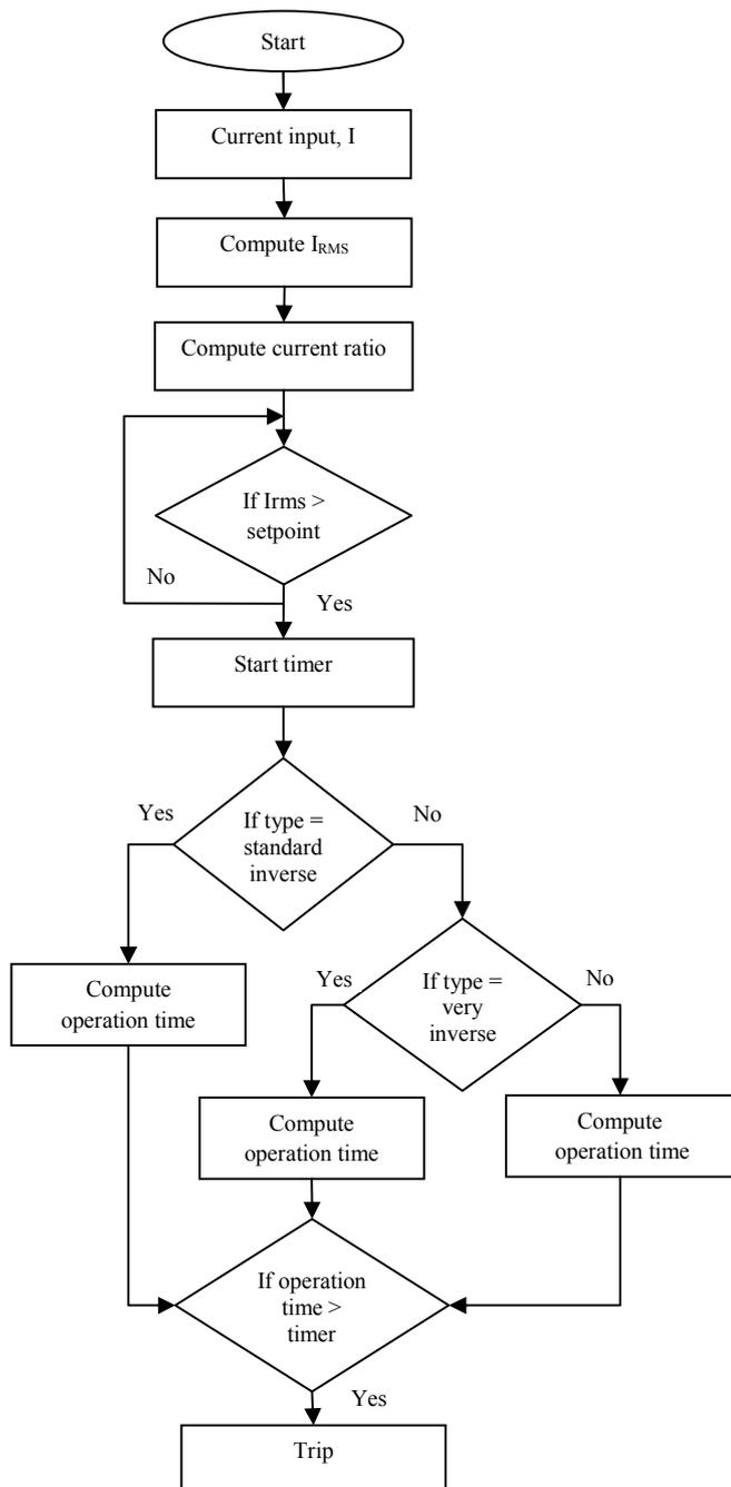
Fig. 2. Flow chart of the protection algorithm for overcurrent relay
