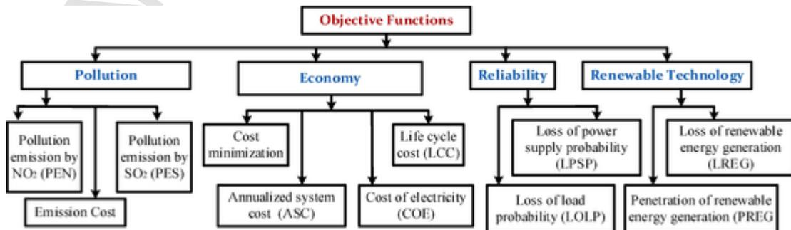
Fig. 8. Key objective functions for the MG optimum operation.
