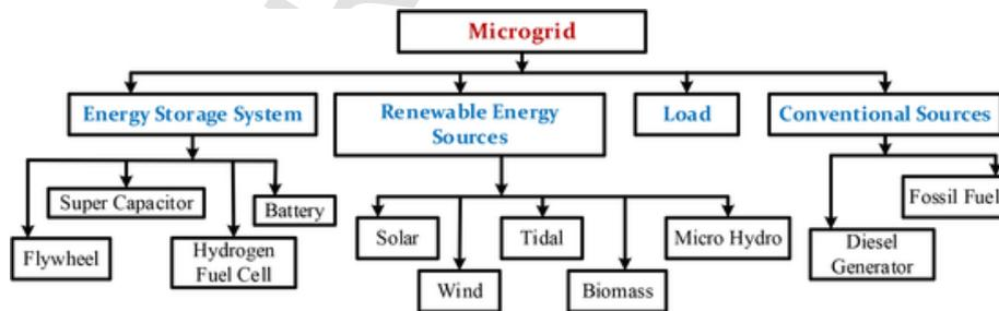
Fig. 6. Type of sources in hybrid MG.
