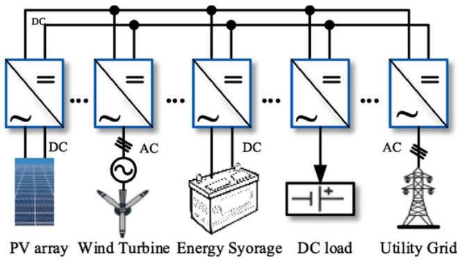
Fig. 5. DC-MG integrated with the bi-directional controller.
