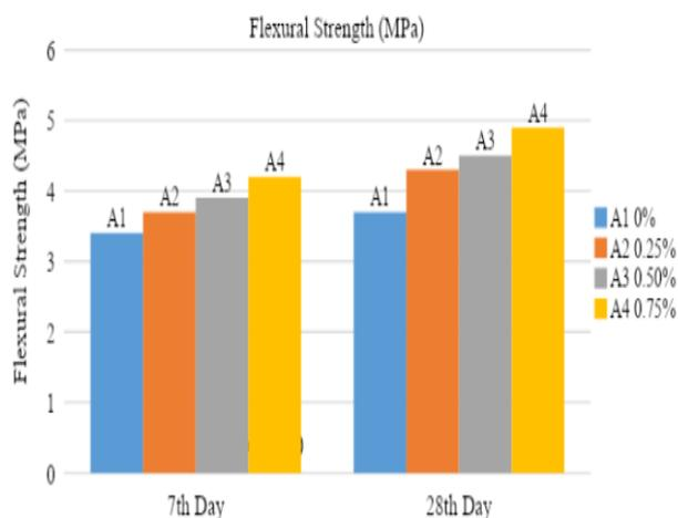
**Fig. 3 Flexural Strength test**
