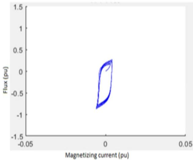
Fig. 6 Hysteresis curve with 200 a injection of GIC
