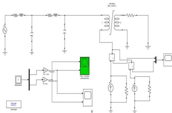
**Fig. 3 Simulation circuit for single-phase saturable transformer**
