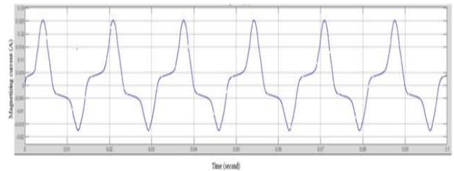
Fig. 10 Magnetizing current with no injection of GIC
