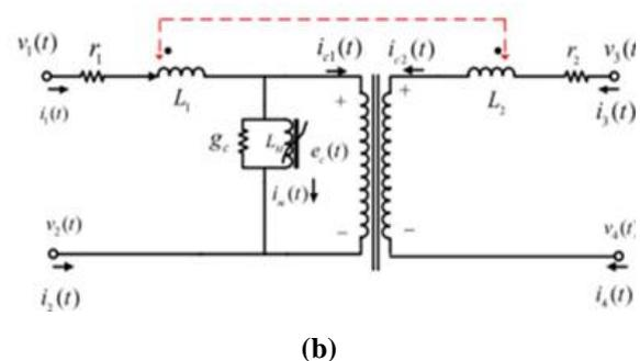
Fig. 2 Single-phase transformer model: (a) two-winding transformer, (b) equivalent circuit [18]
