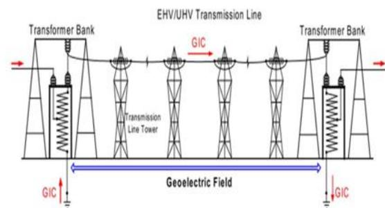
Fig. 1 GIC flow in a power system network [3]
