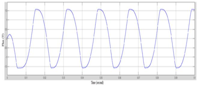
Fig. 8 Flux waveform with 100 a injection of GIC
