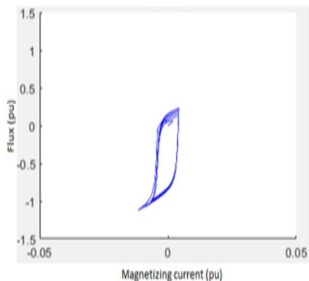
**Fig. 5 Hysteresis curve with 100 a injection of GIC**
