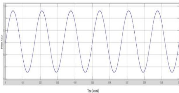
Fig. 7 Flux waveform with no injection of GIC
