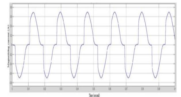
Fig. 12 Magnetizing current with 200 a injection of GIC
