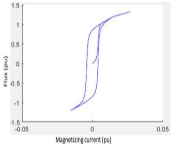
**Fig. 4 Hysteresis curve with no injection of GIC**
