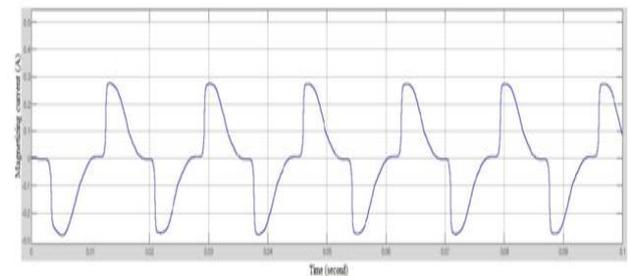
Fig. 11 Magnetizing current with 100 a injection of GIC
