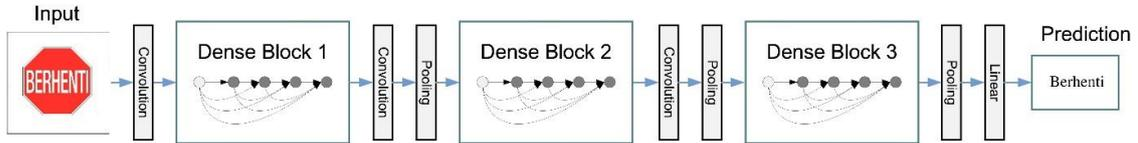
Figure 4. DenseNet model architecture for traffic sign classification.
