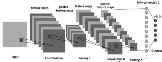
Figure 1. Convolutional Neural Network architecture [23].
