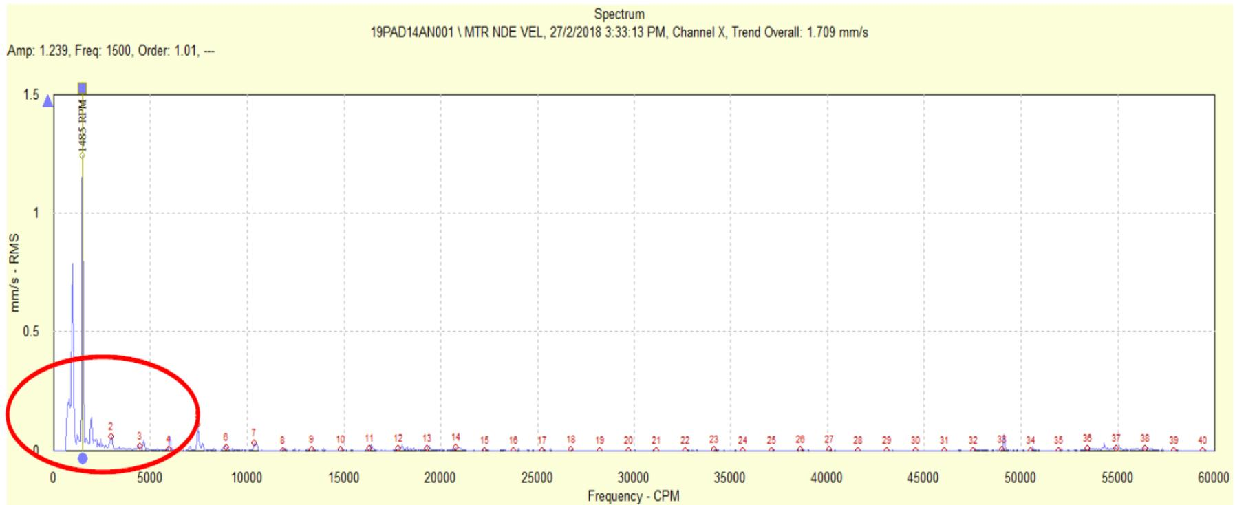
Figure 4.23 CT no.4 Motor NDE Velocity Spectrum after maintenance
