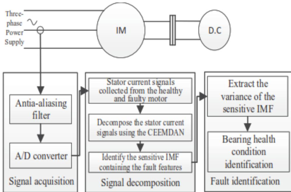
Figure 2.11 The proposed bearing fault detection block diagram [37]
