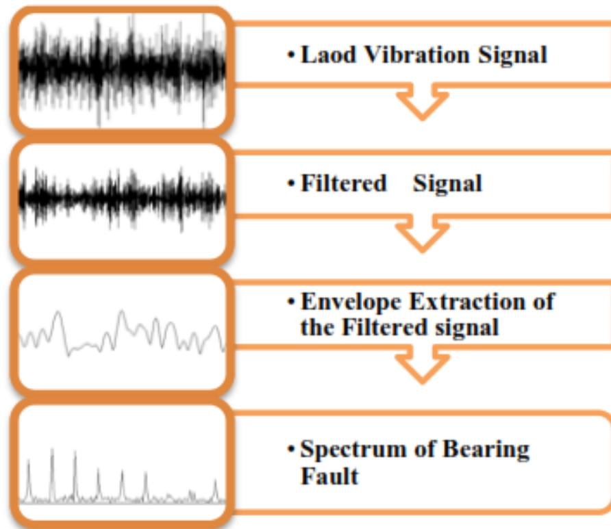
Figure 2.10 Procedure for Envelope Analysis (EA) [35]
