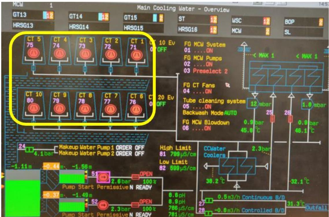
Figure 3.3 CT fan motor in the HMI of the CCPP
