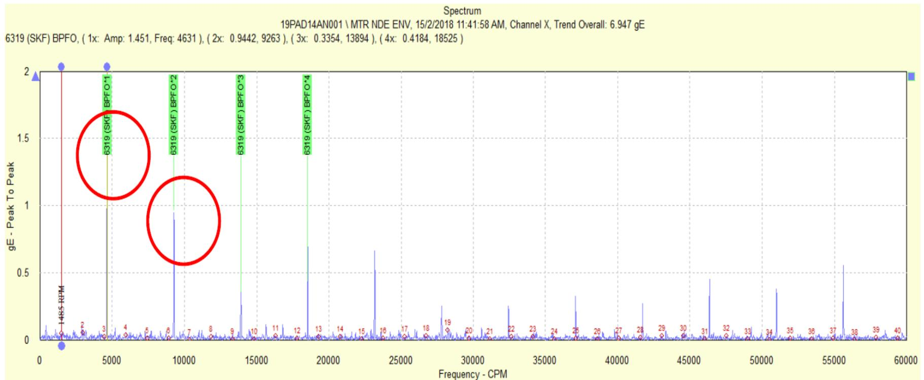
Figure 4.15 CT no.4 Motor NDE Enveloping Spectrum
