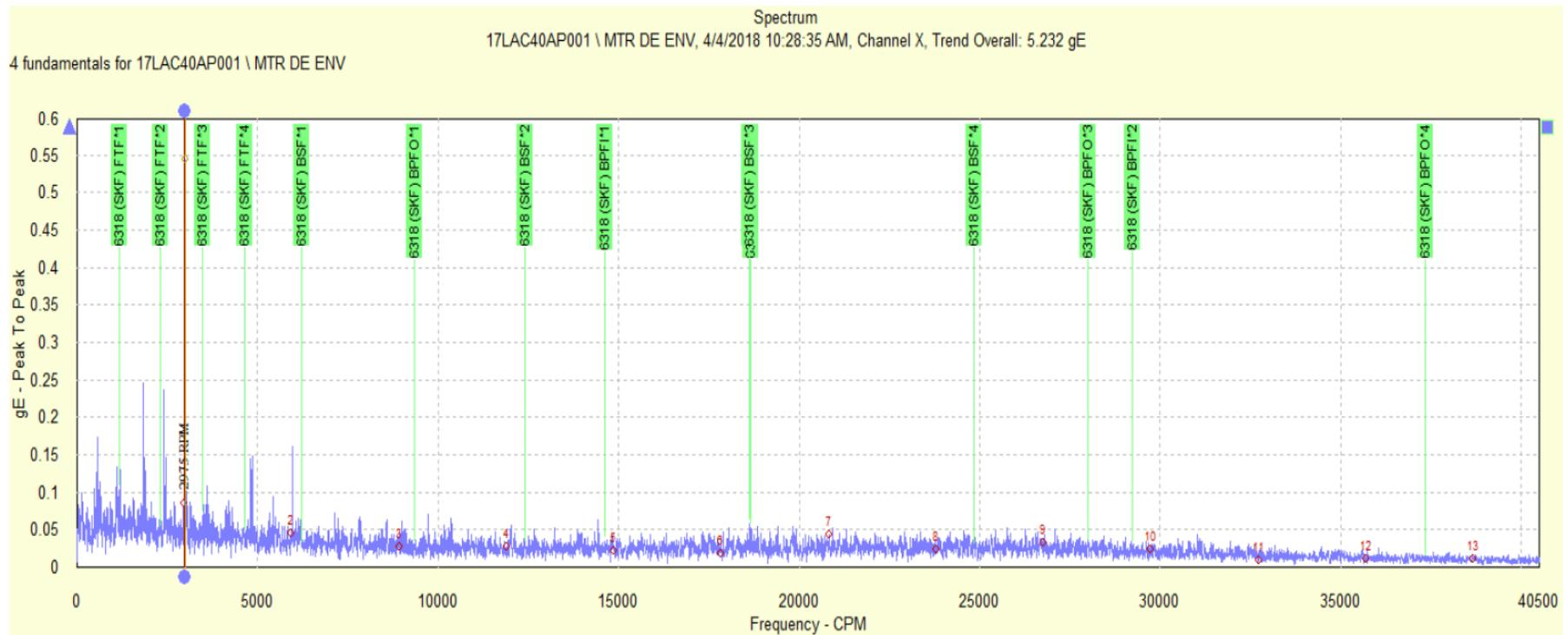
Figure 4.12 LPFW no.4 Motor DE Enveloping Spectrum after maintenance
