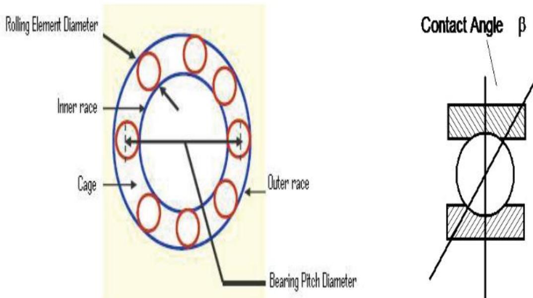
Figure 2.12 Bearing details [39]
