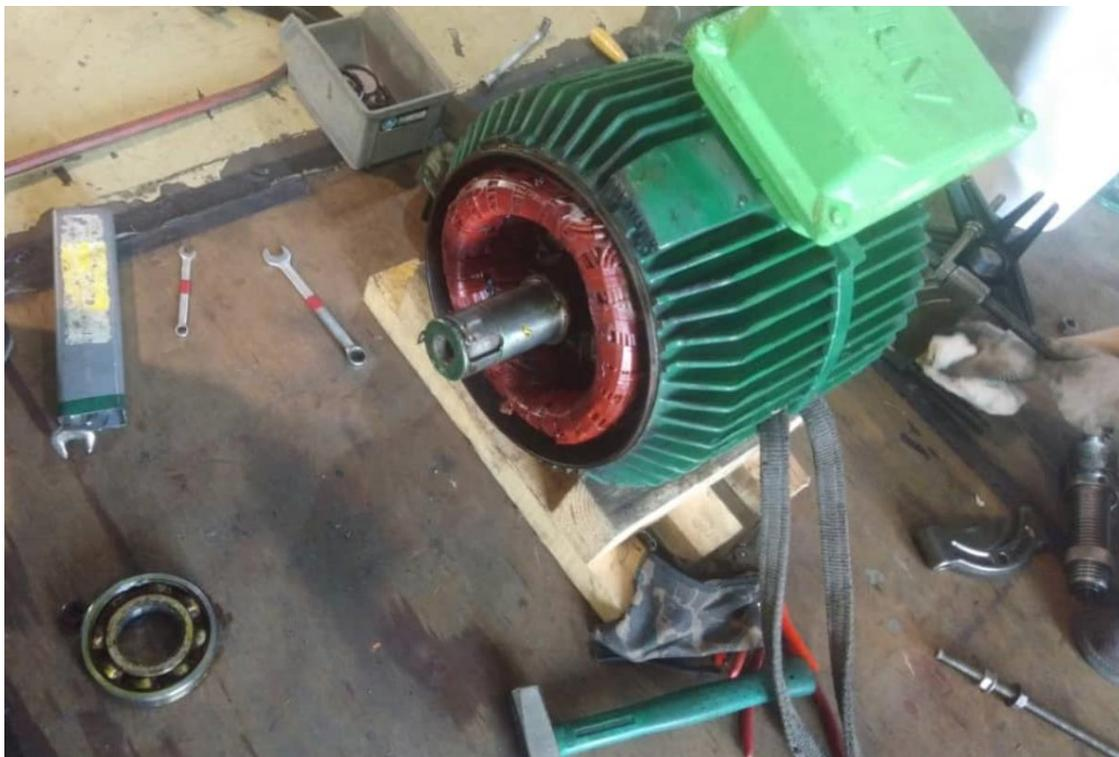
Figure 4.18 CT Fan Motor Bearing Replacement at KLPP Workshop
