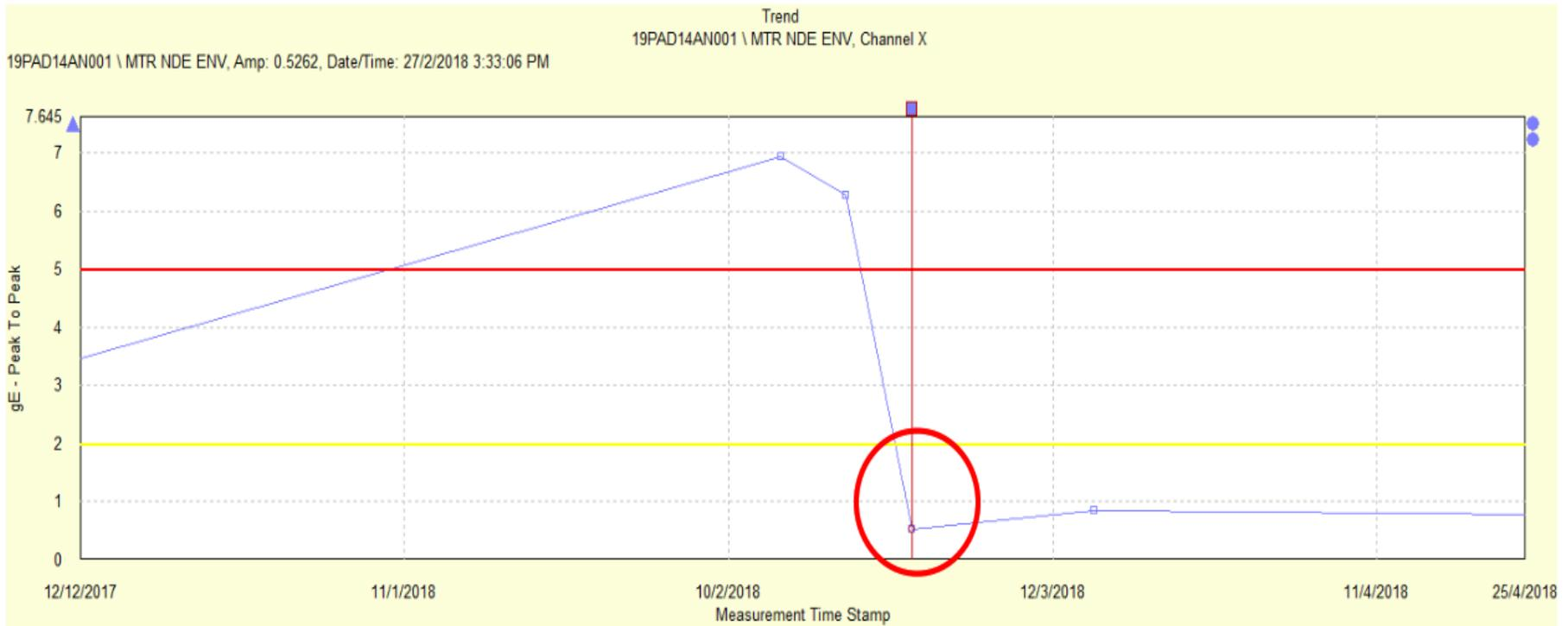
Figure 4.20 CT no.4 Motor NDE Enveloping Trend after maintenance
