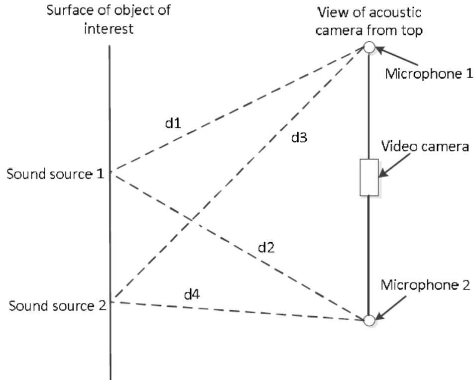
Figure 2.5 Sample view of acoustic camera from top, schematic illustration of principle of acoustic camera [22]
