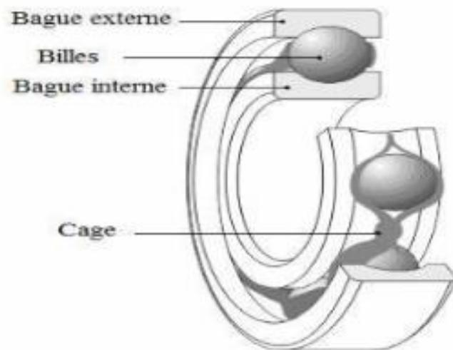
Figure 2.9 The component of bearing [34]
