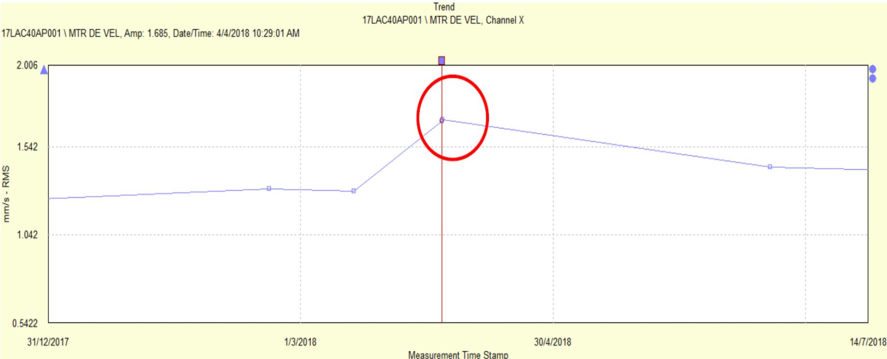
Figure 4.13 LPFW no.4 Motor DE Velocity Trend after maintenance
