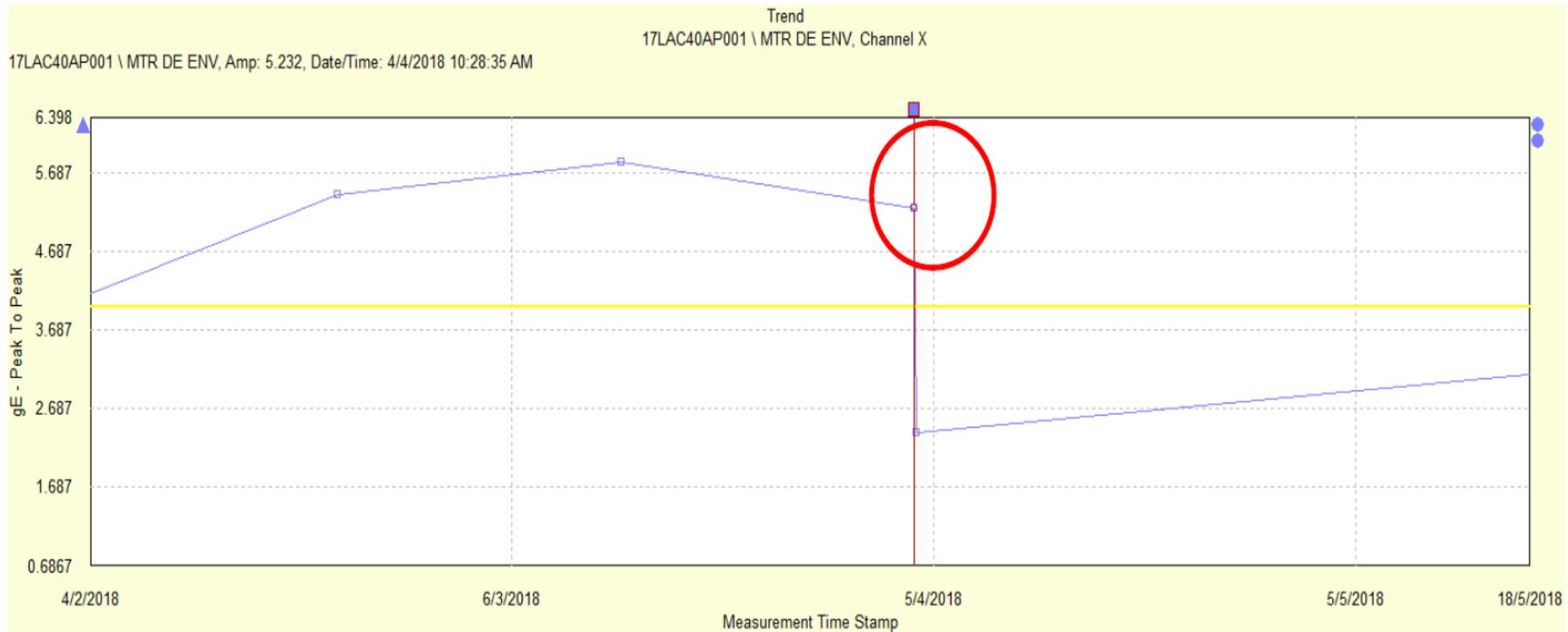
Figure 4.4 LPFW no.4 Motor DE Enveloping Trend
