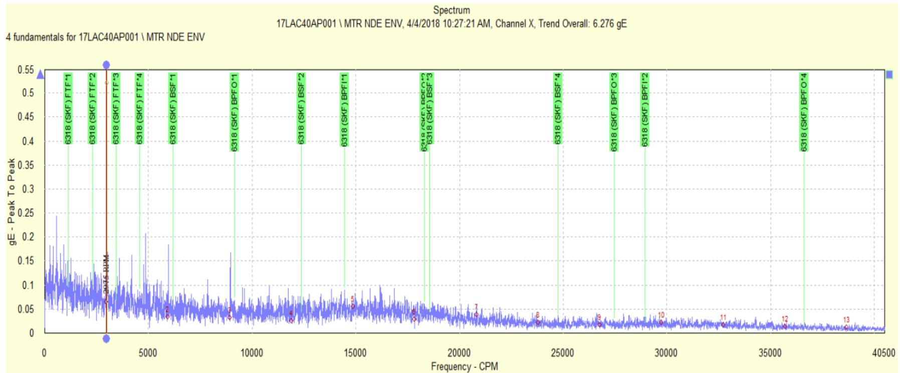
Figure 4.2 LPFW no.4 Motor NDE Enveloping Spectrum
