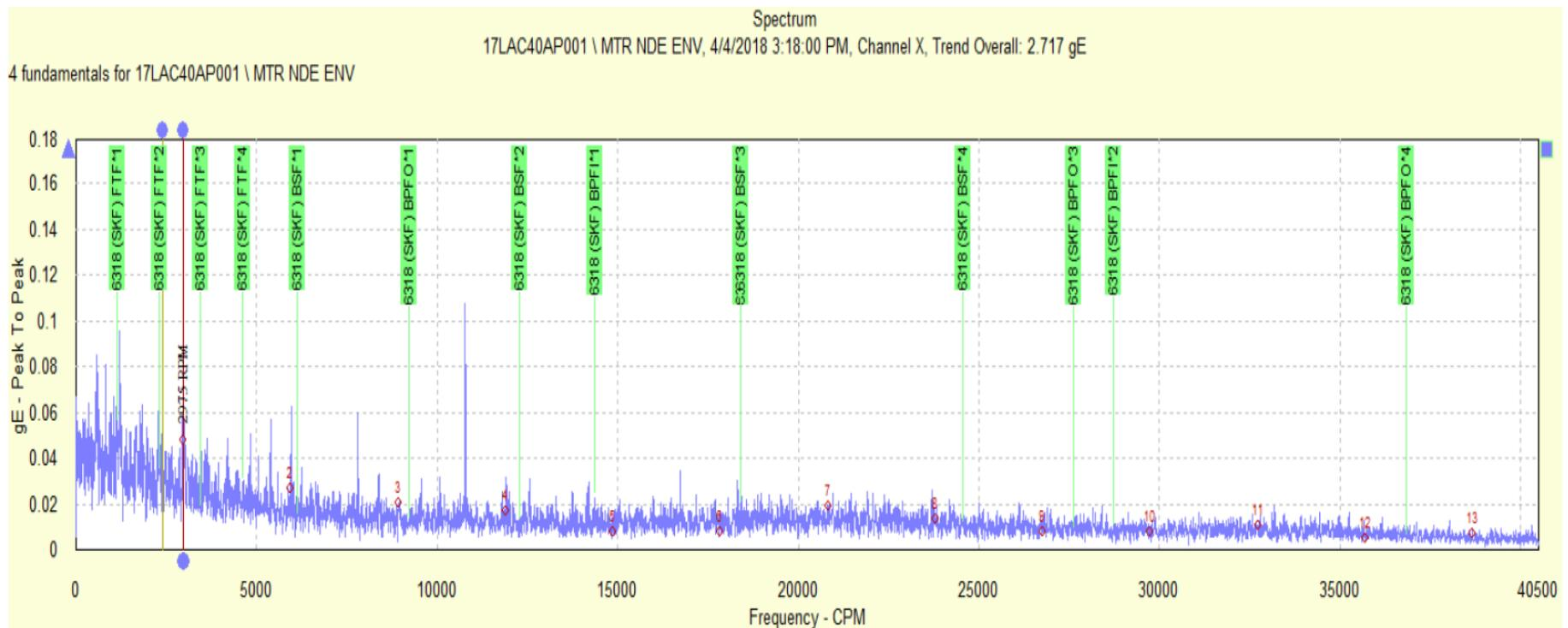
Figure 4.9 LPFW no.4 Motor NDE Enveloping Spectrum after maintenance
