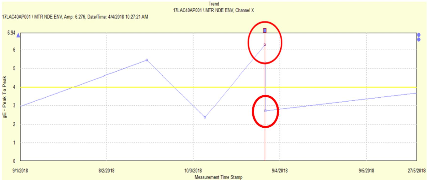
Figure 4.8 LPFW no.4 Motor NDE Enveloping Trend after maintenance
