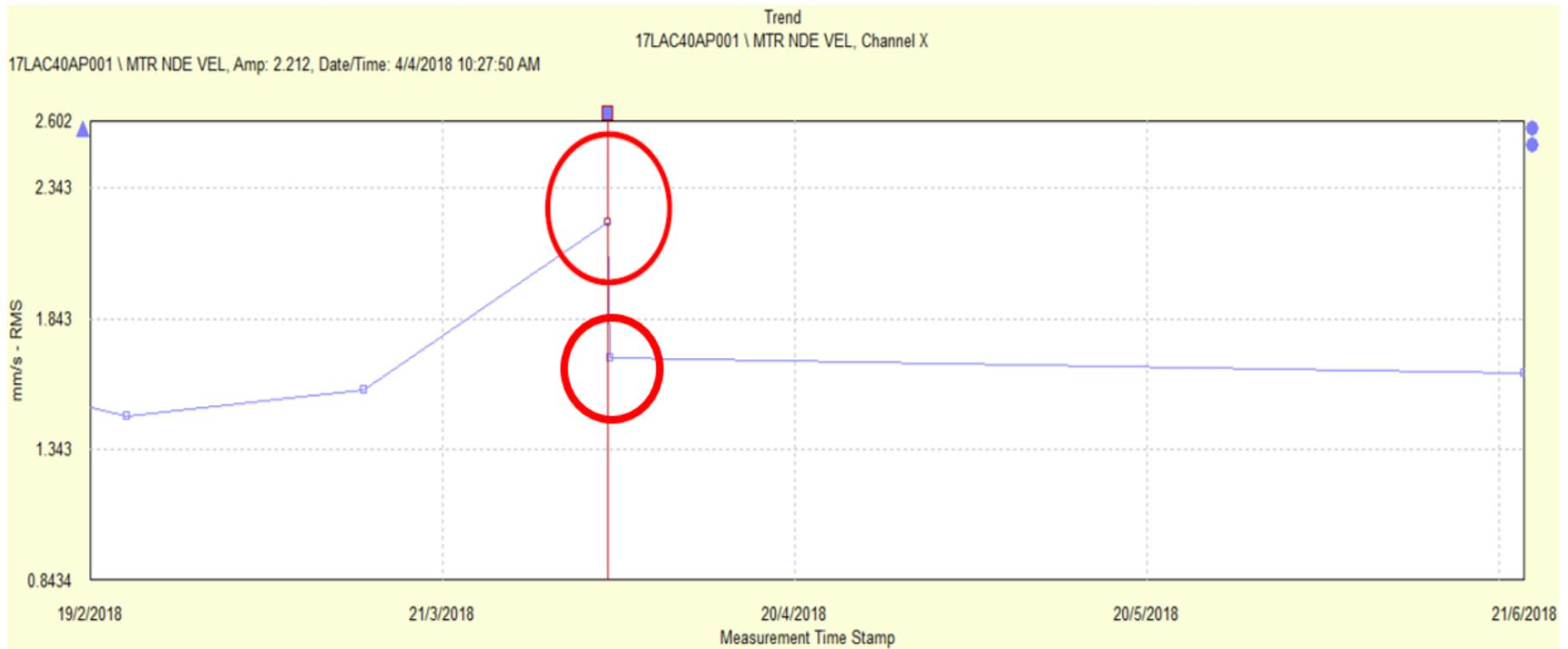
Figure 4.10 LPFW no.4 Motor NDE Velocity Trend after maintenance
