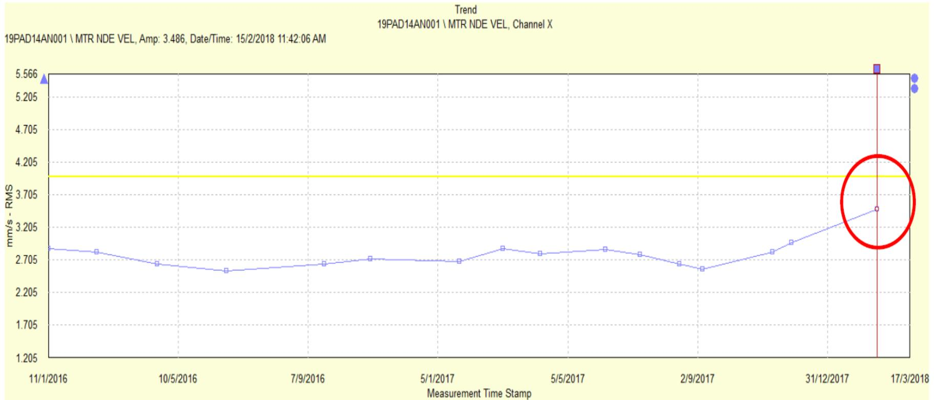
Figure 4.16 CT no.4 Motor NDE Velocity Trend
