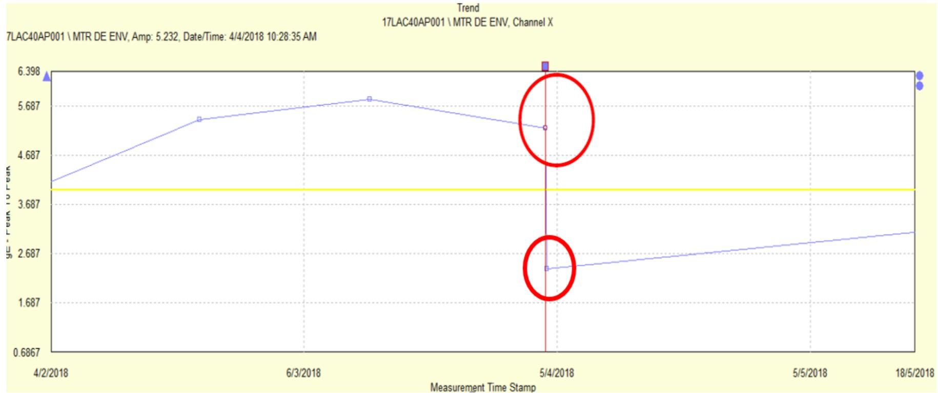
Figure 4.11 LPFW no.4 Motor DE Enveloping Trend after maintenance
