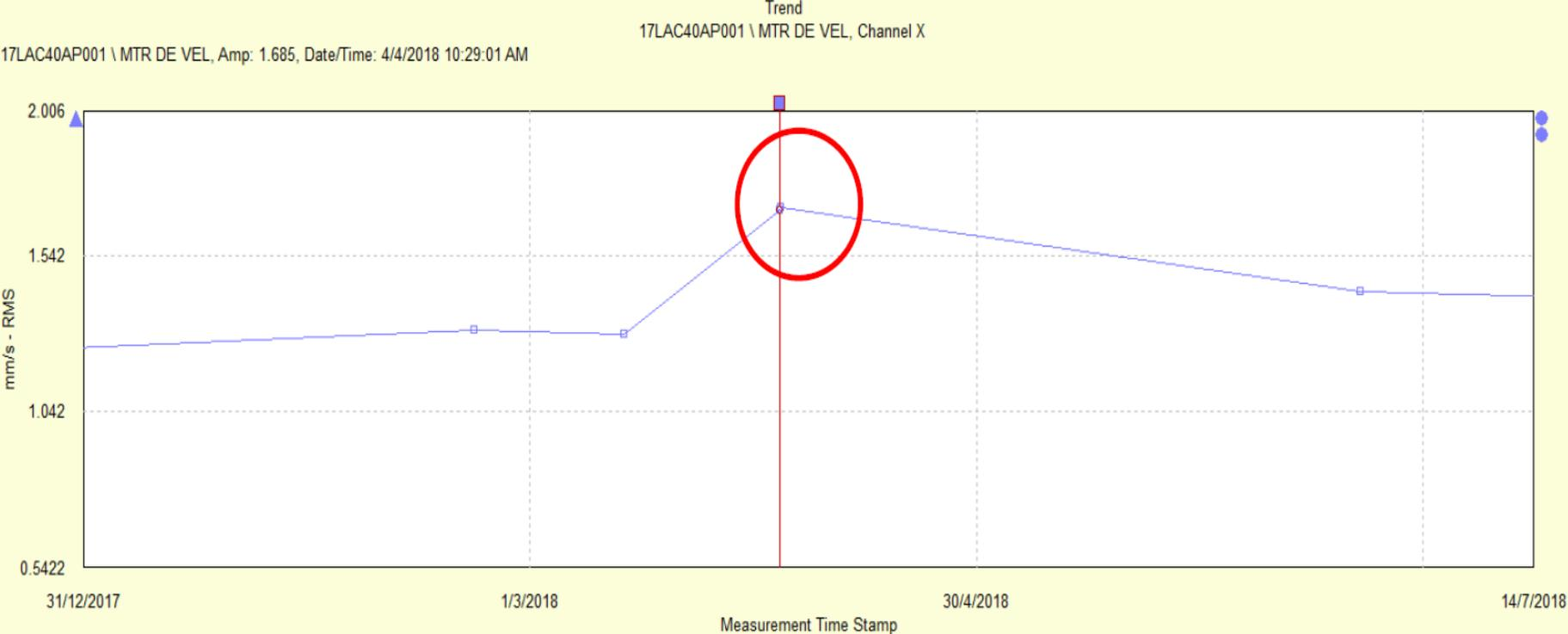
Figure 4.6 LPFW no.4 Motor DE Velocity Trend
