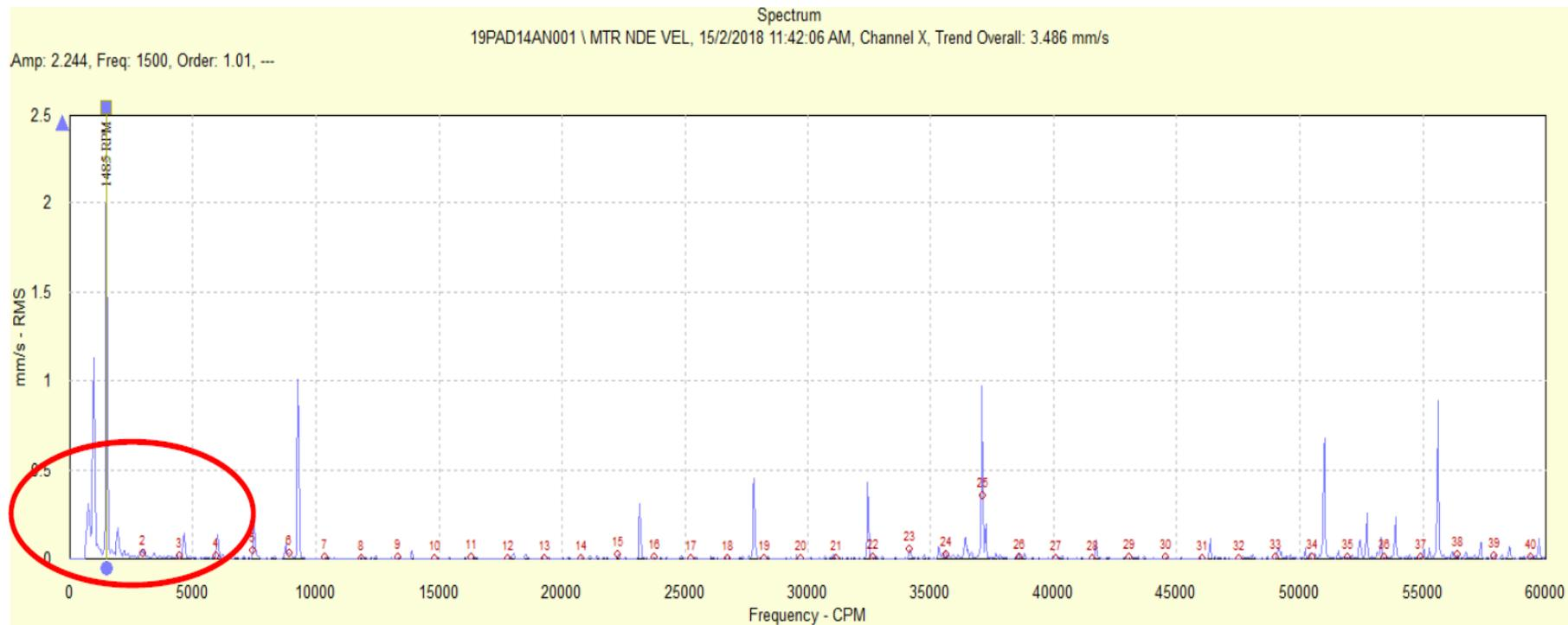
Figure 4.17 CT no.4 Motor NDE Velocity Spectrum Amplitude
