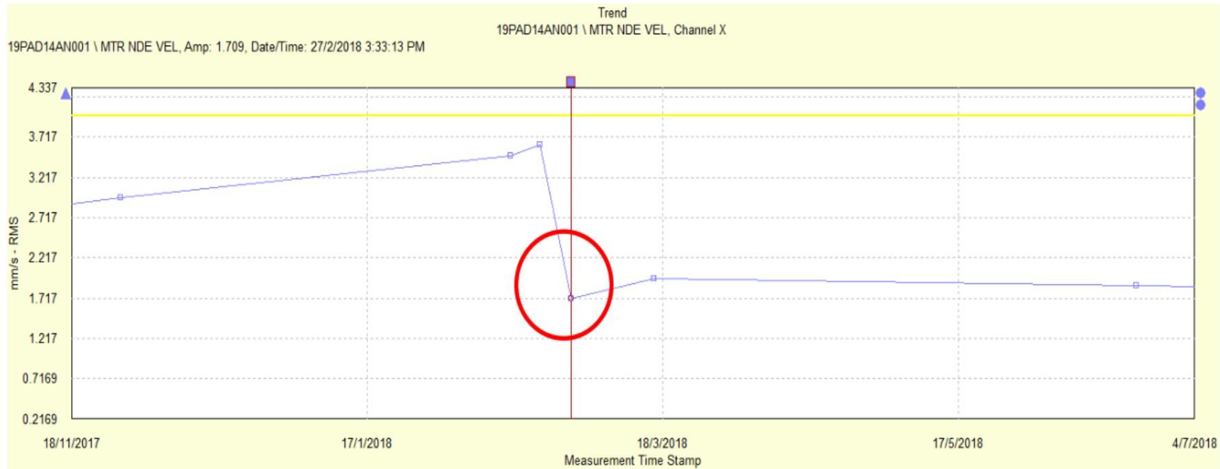
Figure 4.22 CT no.4 Motor NDE Velocity Trend after maintenance
