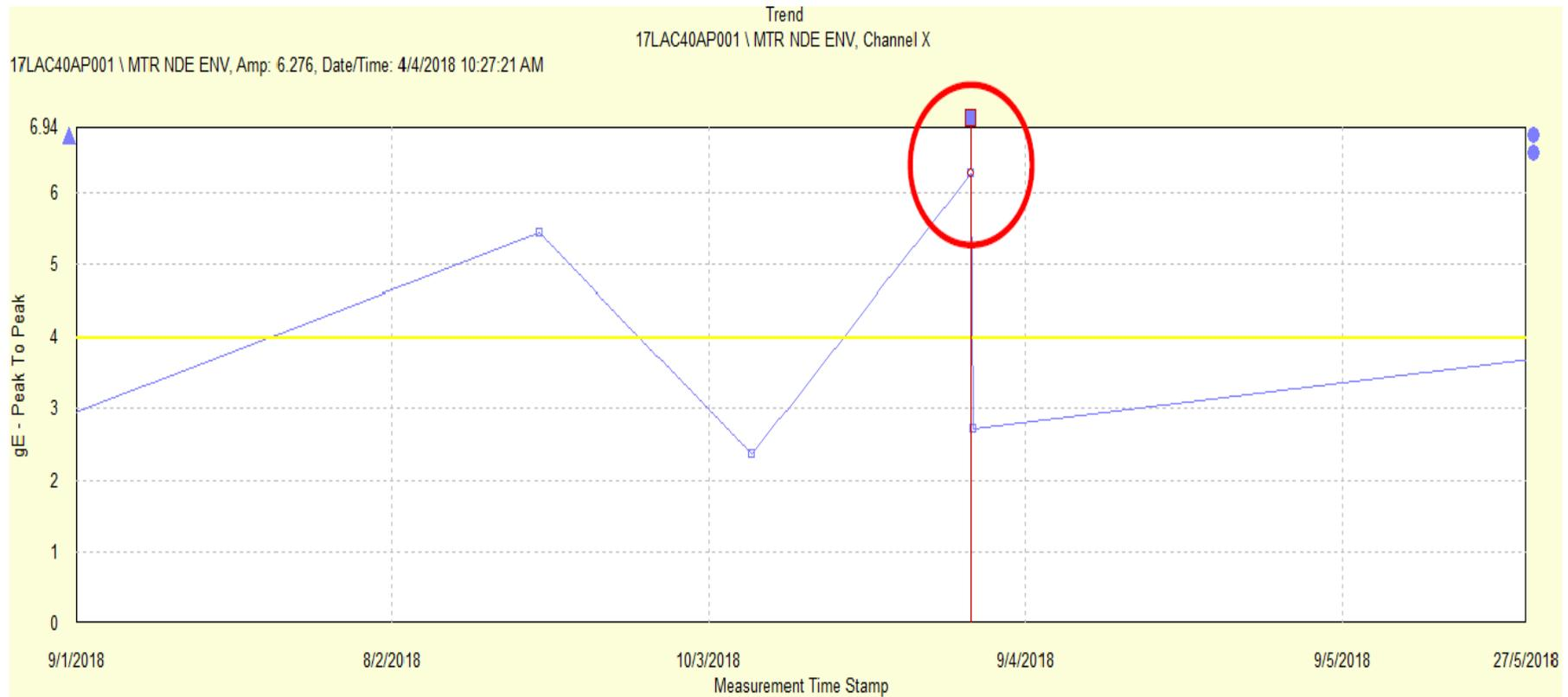
Figure 4.1 LPFW no.4 Motor NDE Enveloping Trend
