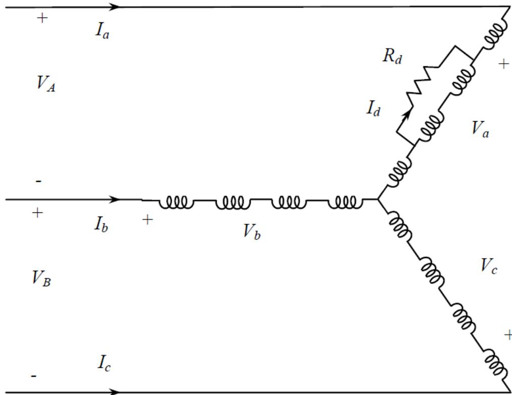
Figure 2.3 Sample Stator Winding of an Induction Motor with Simulated Deterioration [9]
