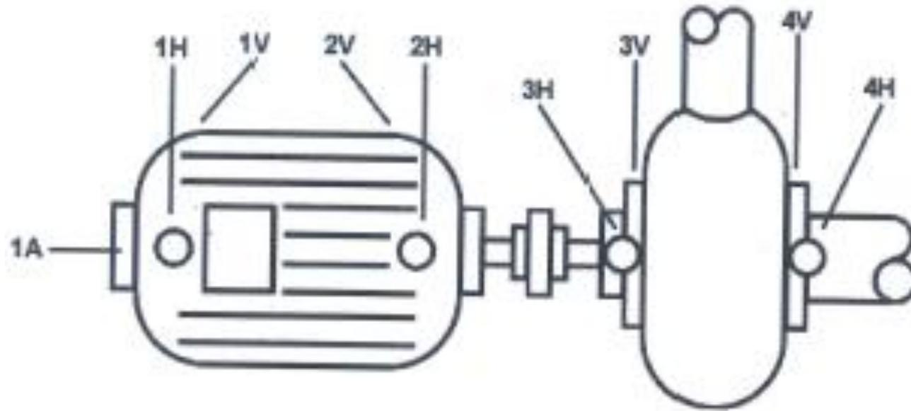
Figure 3.7 Measurement identifications for horizontal motor and pump [47]
