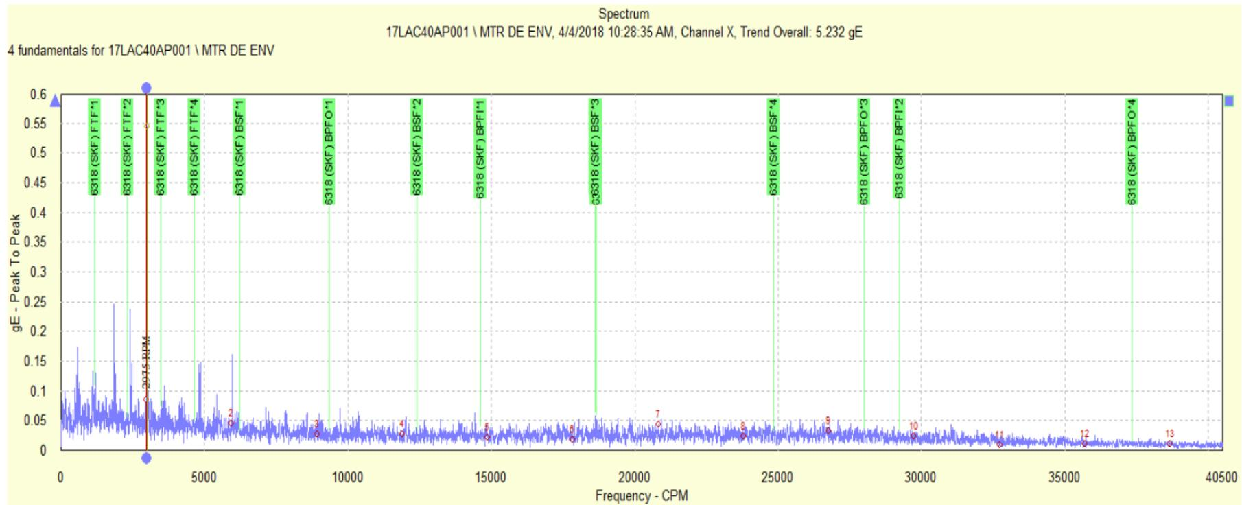
Figure 4.5 LPFW no.4 Motor DE Enveloping Spectrum
