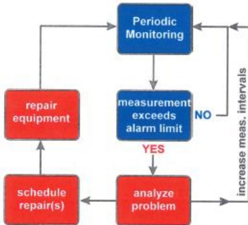
Figure 3.6 Simple flow work for predictive maintenance
