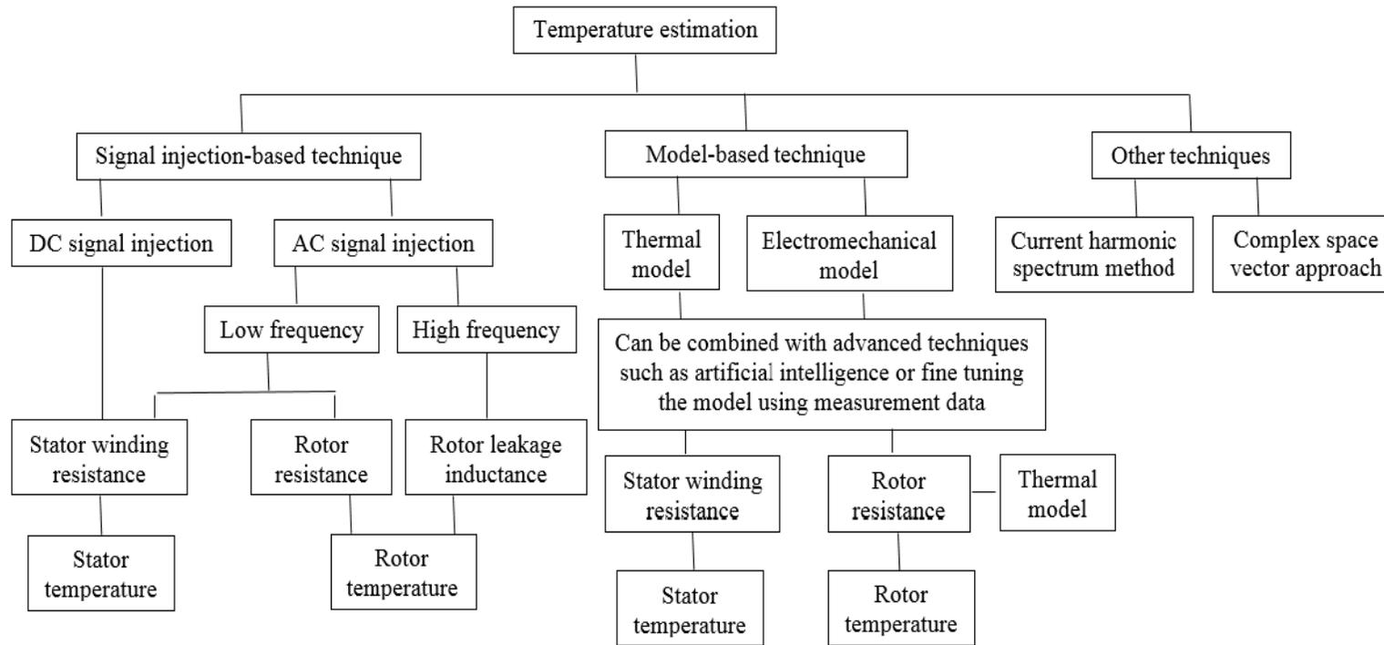
Figure 2.4 Sample motor temperature estimation techniques [17]
