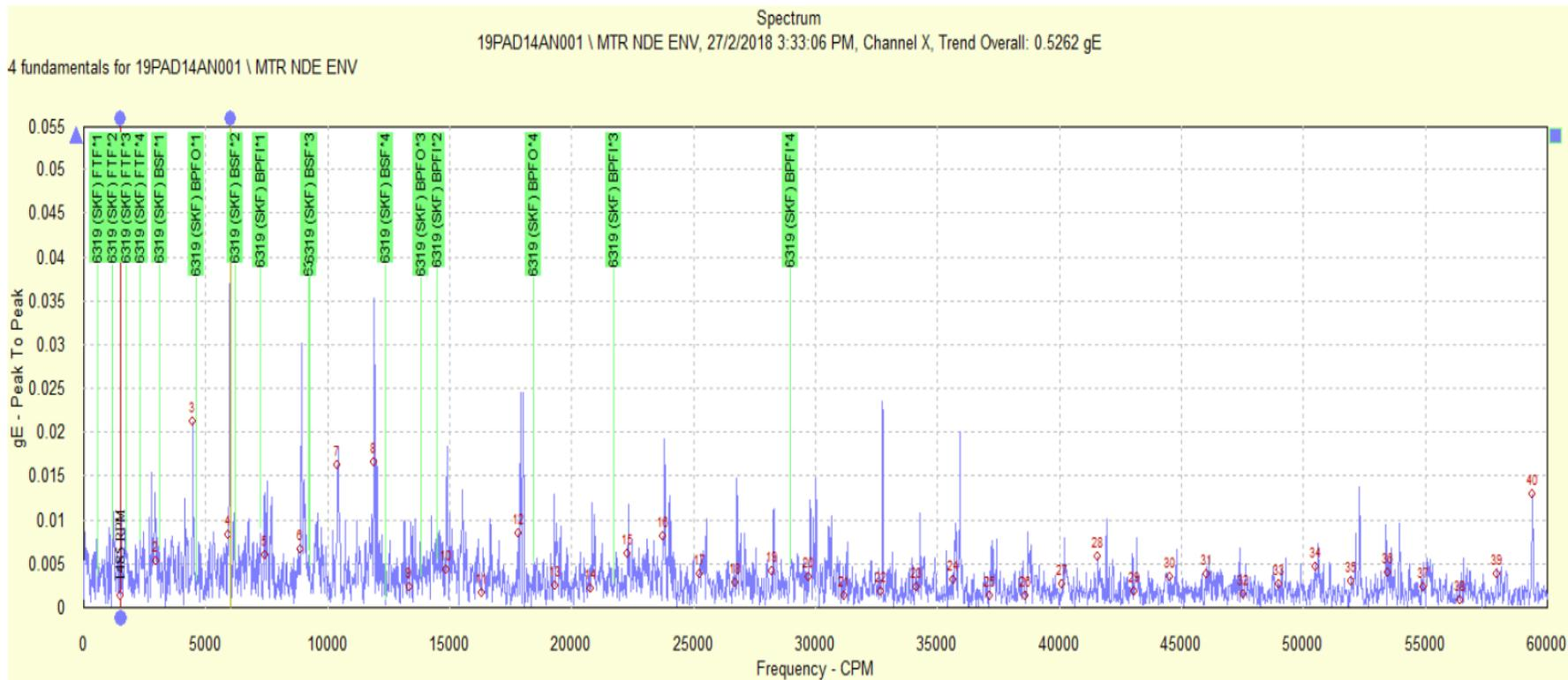
Figure 4.21 CT no.4 Motor NDE Enveloping Spectrum after maintenance
