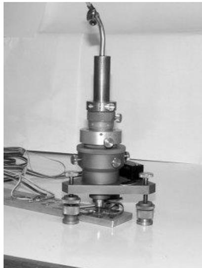
Figure 2.12 Hole drilling apparatus [116].
