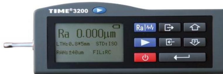
Figure 3.9 TR200 surface roughness measurer.
