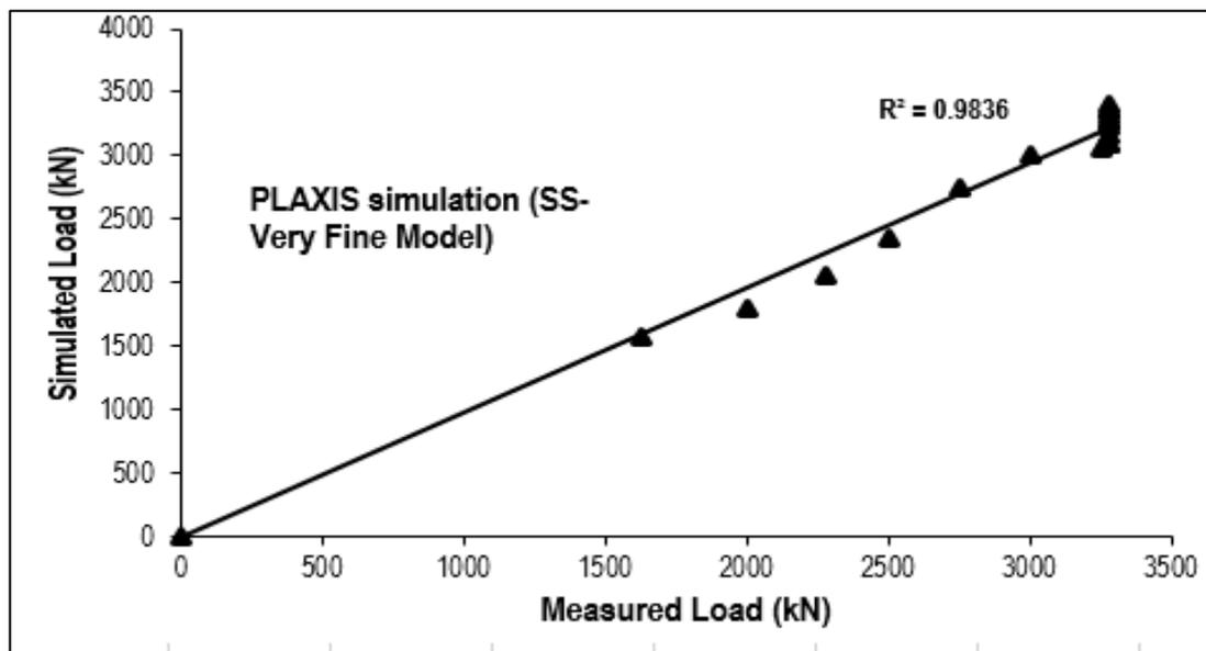
Figure 4.14. The result of  $R^2$  for the simulated load versus measured load for the single bored pile in clayey soil using Soft Soil model in Very Fine mesh by the PLAXIS simulation.
