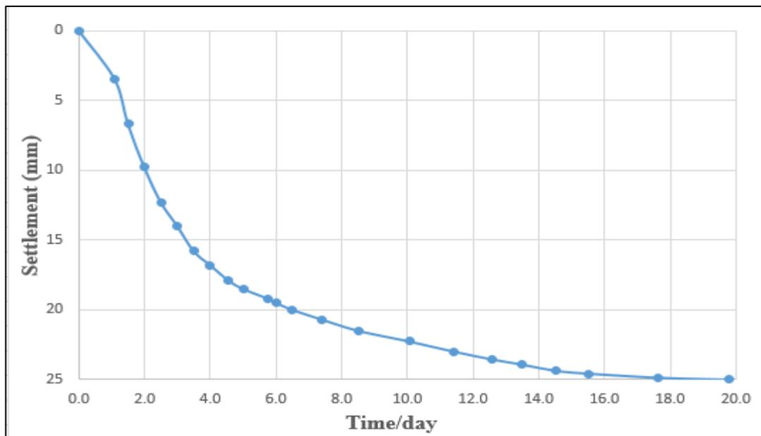
Figure 4.24. The relationship between settlement and time for the mid pile tip point of the group bored piles subjected to pile spacing of 3D in the clayey soil under the PLAXIS simulation.
