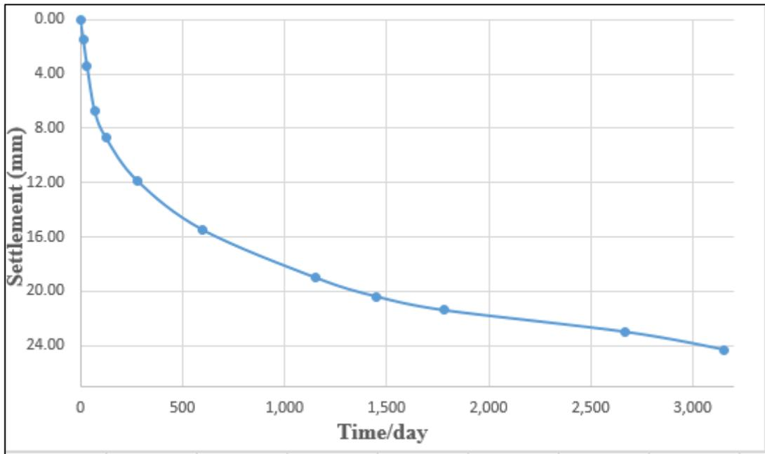
Figure 4.35. The relationship between settlement and time for the mid pile tip point of the group bored piles subjected to soil cohesion of 20 kPa in the clayey soil under the PLAXIS simulation.
