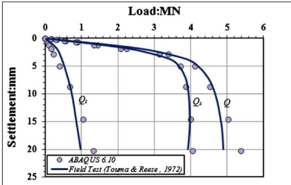
Figure 2.5. Comparison between field test data and numerical simulation of Load-Settlement curves of single bored pile in soil (Tosini et al., 2010).
