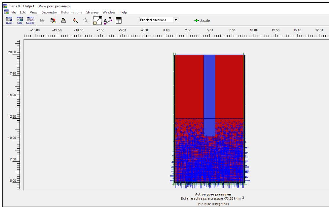
Figure 3.6. Simulation of pore water pressure distribution of the single bored pile in clayey soil.
