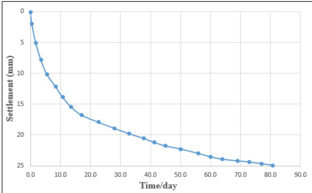
Figure 4.20. The relationship between settlement and time for the mid pile tip point of the group bored piles subjected to pile diameter of 1.3 m in the clayey soil under the PLAXIS simulation.
