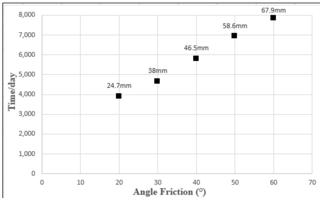
Figure 4.41. The relationship between time and soil angle friction for the mid pile tip point of the group bored piles in the clayey soil under the PLAXIS simulation.
