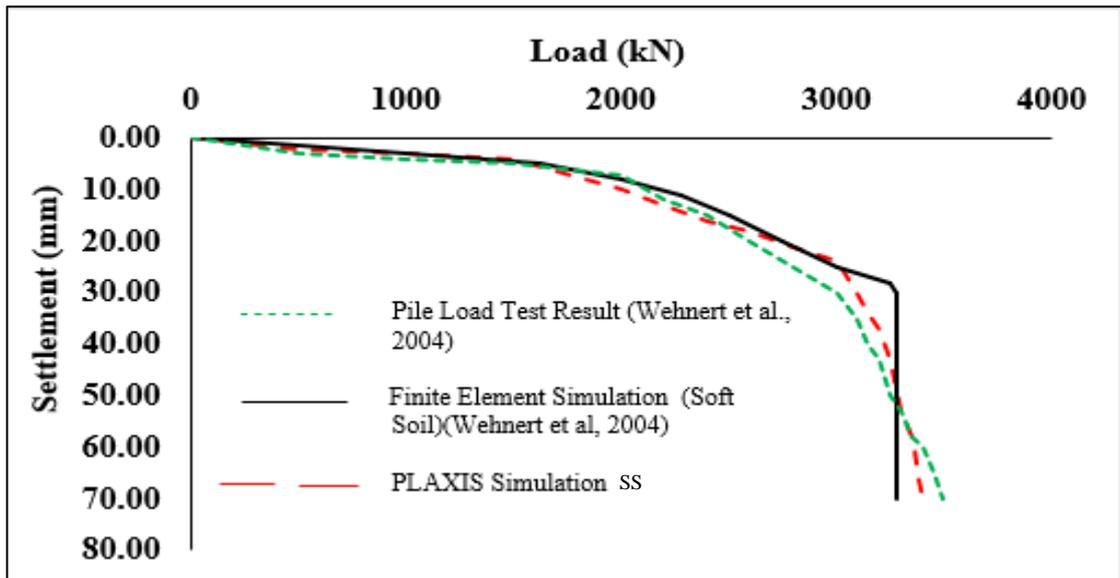
Figure 4.6. Load-settlement behaviour of single bored pile in clayey soil using SS model for Very Fine mesh PLAXIS simulation in comparison to the measured and simulated ones from Wehnert & Vermeer (2004).
