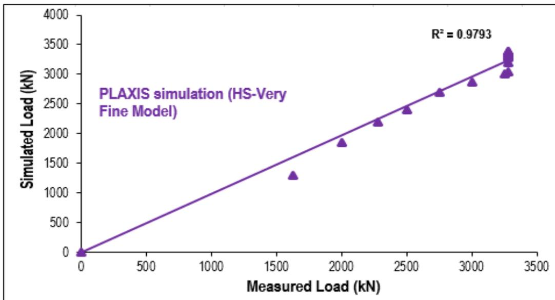
Figure 4.12. The result of  $R^2$  for the simulated load versus measured load for the single bored pile in clayey soil using Hard Soil model in Very Fine mesh by the PLAXIS simulation.
