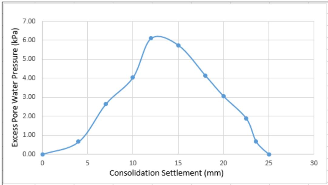
Figure 4.23. The relationship between excess pore water pressure and consolidation settlement for the mid pile tip point of the group bored piles subjected to 50 kPa applied pressure, pile diameter of 1.3 m and pile spacing of 3D in the clayey soil under the PLAXIS simulation.
