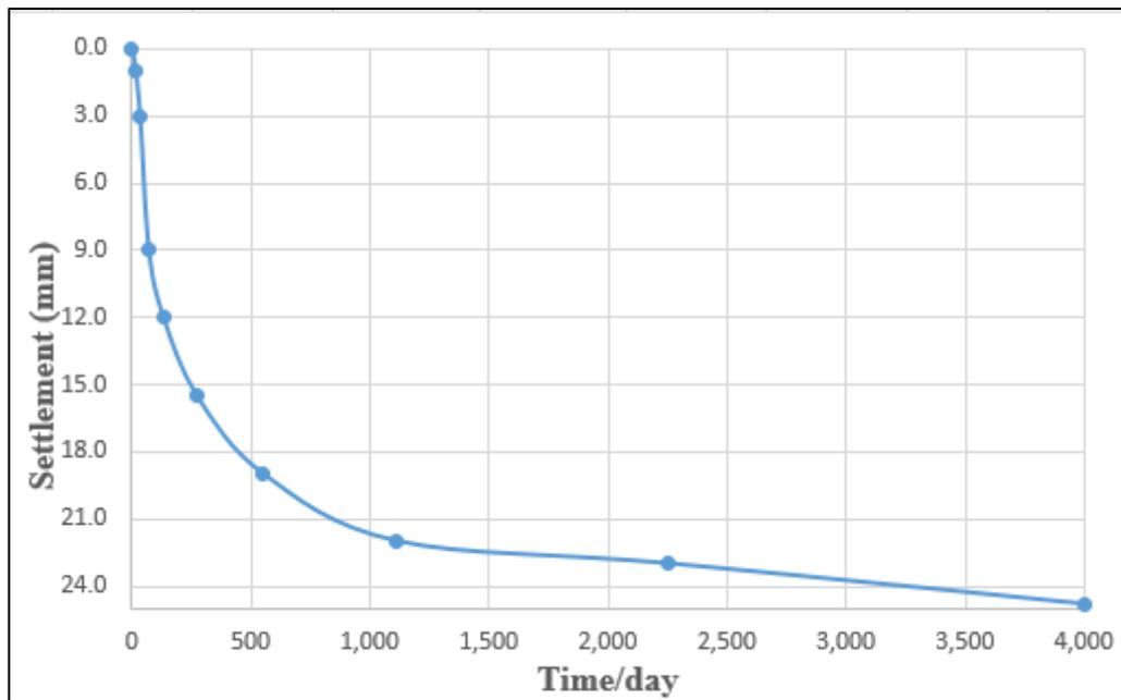
Figure 4.30. The relationship between settlement and time for the mid pile tip point of the group bored piles subjected pile slope ratio of 1:2 in the clayey soil under the PLAXIS simulation.
