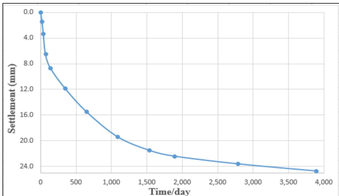
Figure 4.39. The relationship between settlement and time for the mid pile tip point of the group bored piles subjected to soil angle of internal friction of 20° in the clayey soil under the PLAXIS simulation.
