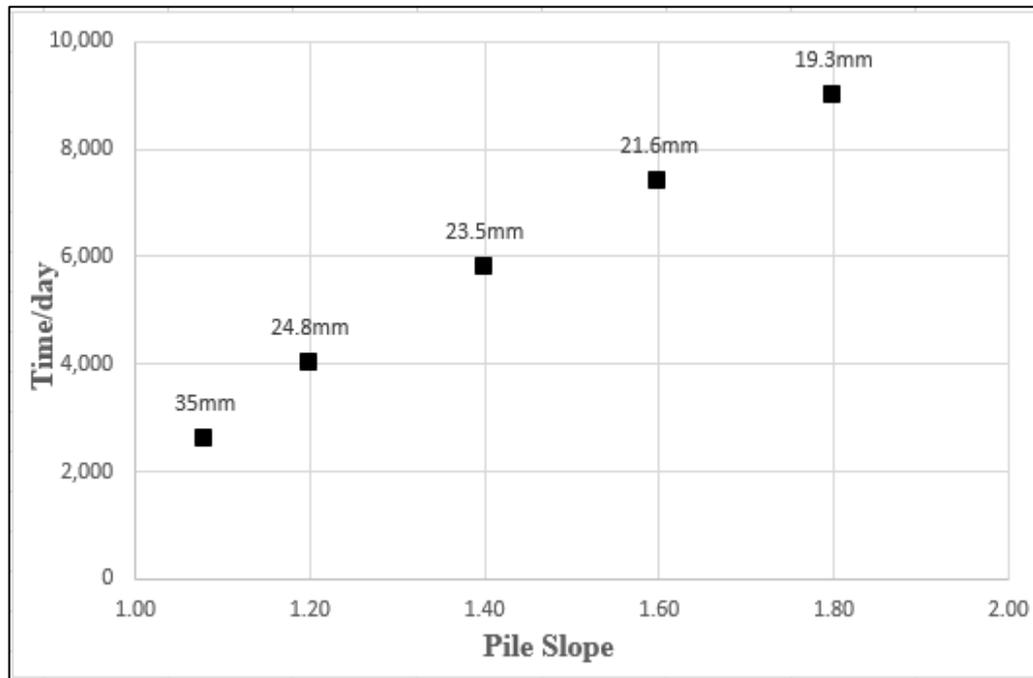
Figure 4.32. The relationship between time and pile slope for the mid pile tip point of the group bored piles in clayey soil under the PLAXIS simulation.
