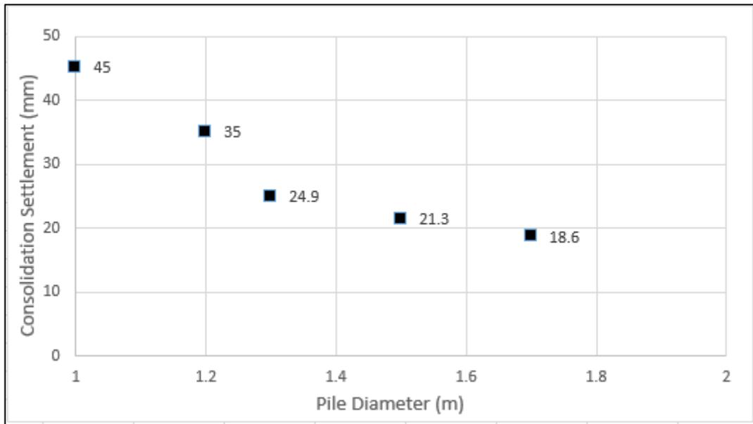
Figure 4.21. The relationship between consolidation settlement for the mid pile tip point of the group bored piles and pile diameter in the clayey soil under the PLAXIS simulation.
