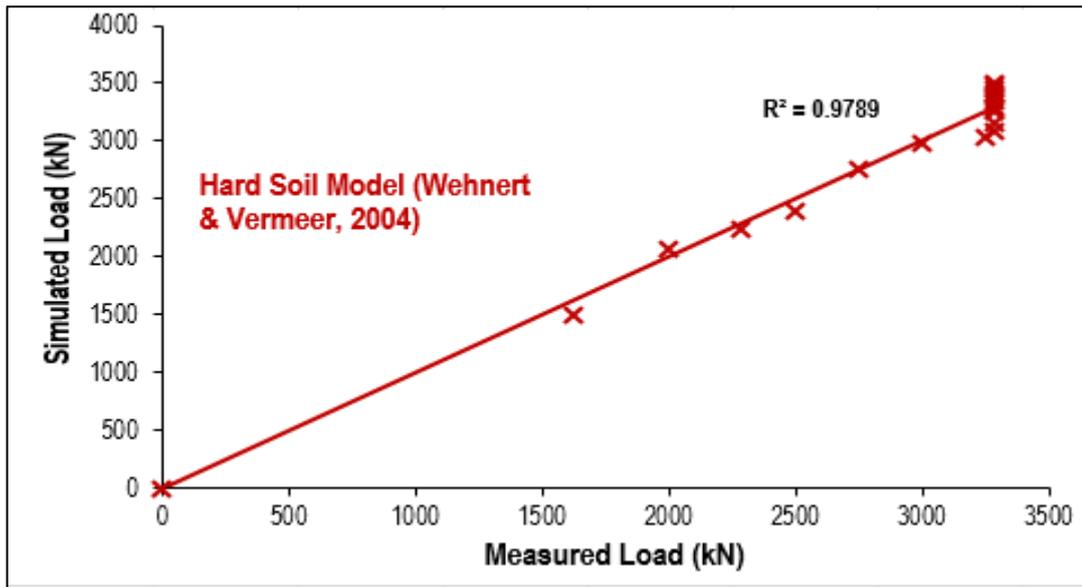
Figure 4.11. The result of  $R^2$  for the simulated load versus measured load for the single bored pile in clayey soil using Hard Soil model in Very Fine mesh by Wehnert and Vermeer (2004).
