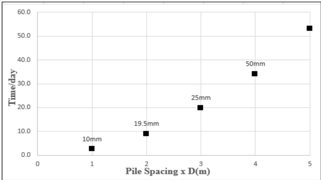
Figure 4.26. The relationship between time and pile spacing for the mid pile tip point of the group bored piles in the clayey soil under the PLAXIS simulation.
