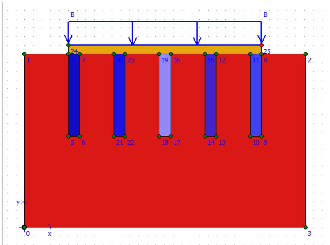
Figure 4.27. The group bored piles arrangement in the clayey soil with zero slope ratio.
