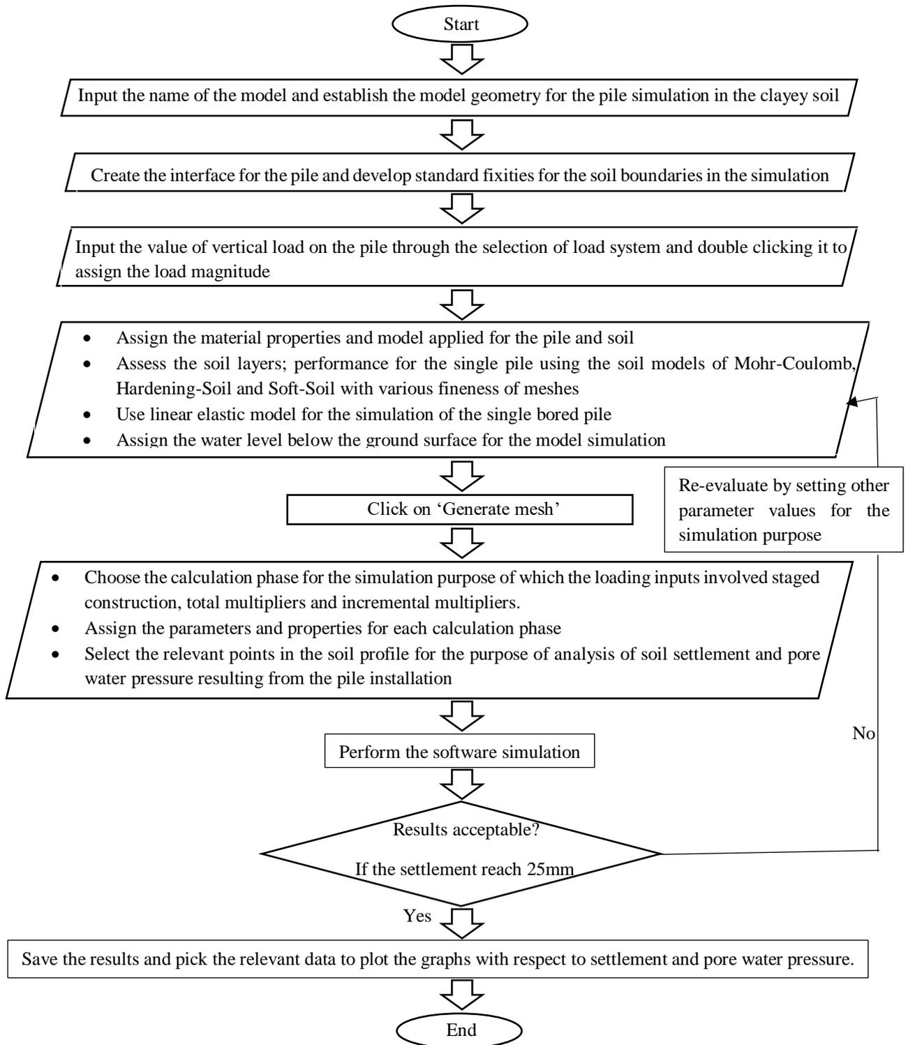
Figure 3.2. Flowchart of methodology of PLAXIS simulation on the bored piles.
