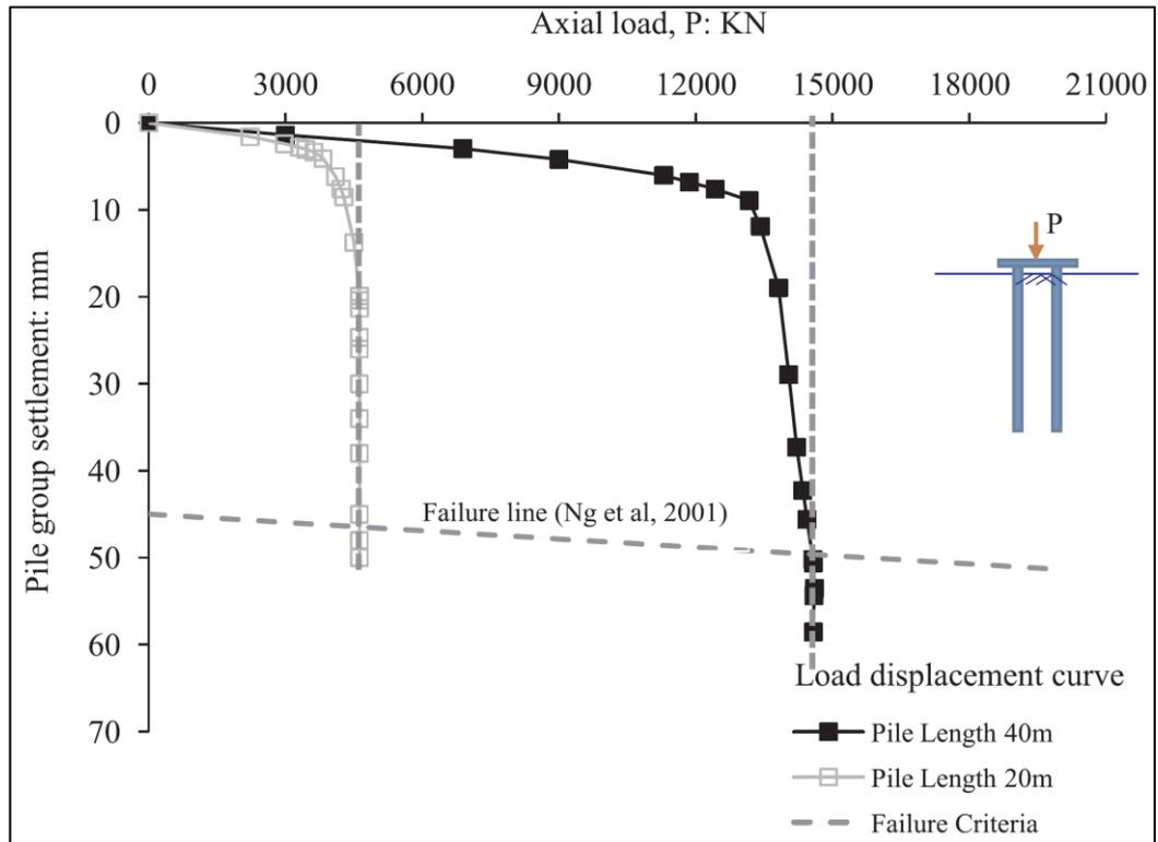
Figure 2.9. Computed load settlement curves for pile group in soft clay (Shakeel and Ng, 2018).
