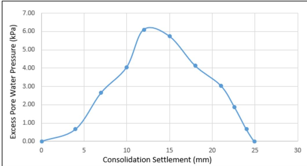
Figure 4.19. The relationship between excess pore water pressure and consolidation settlement for the mid pile tip point of the group bored piles subjected to 50 kPa applied pressure and pile diameter of 1.3 m in the clayey soil under the PLAXIS simulation.
