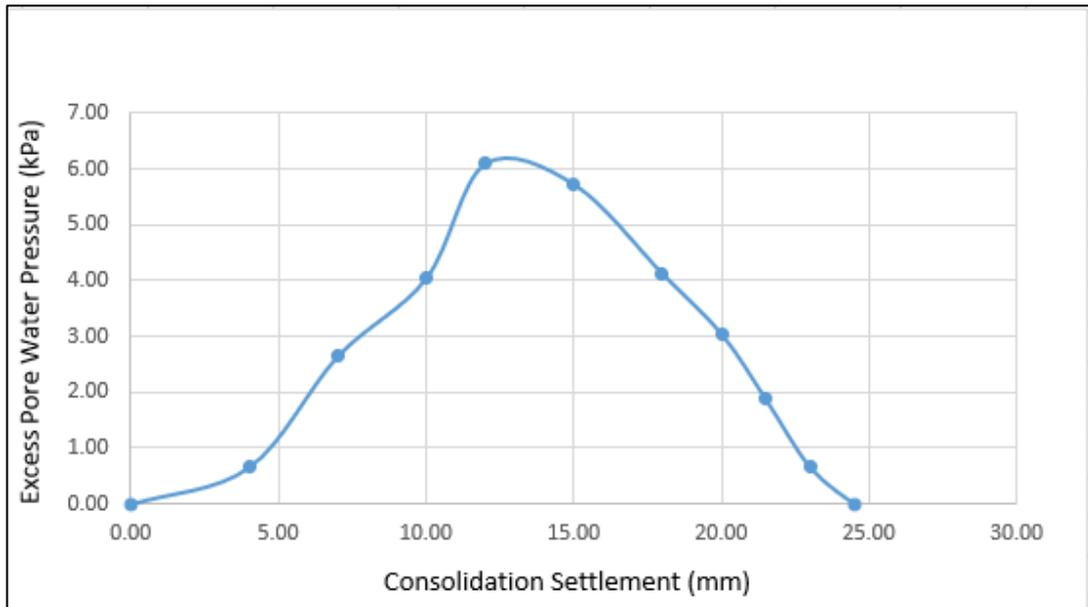
Figure 4.15. The relationship between excess pore water pressure and consolidation settlement for the mid pile tip point of the group bored piles subjected to 50 kPa applied pressure in the clayey soil under the PLAXIS simulation.
