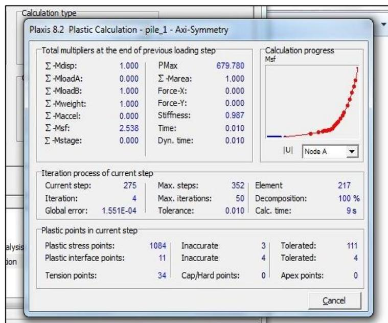
Figure 3.9. Calculation in PLAXIS based on the 3 phases of loading input.
