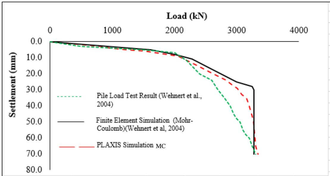
Figure 4.2. Load-settlement behaviour of single bored pile in clayey soil using MC model for Very Fine mesh PLAXIS simulation in comparison to the measured and simulated ones from Wehnert and Vermeer (2004).
