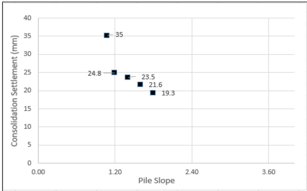
Figure 4.31. The relationship between consolidation settlement for the mid pile tip point of the group bored piles and pile slope ratio in clayey soil under the PLAXIS simulation.
