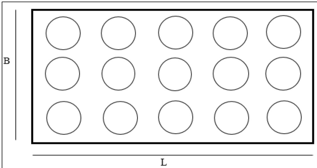
Figure 3.11. Plan view of the foundation designed in 5 × 3 group bored pile arrangement (Note: For the pile cap,  $B$  = Breadth = 9.1 m;  $L$  = Length = 20.8 m,  $H$  = Thickness = 1 m).
