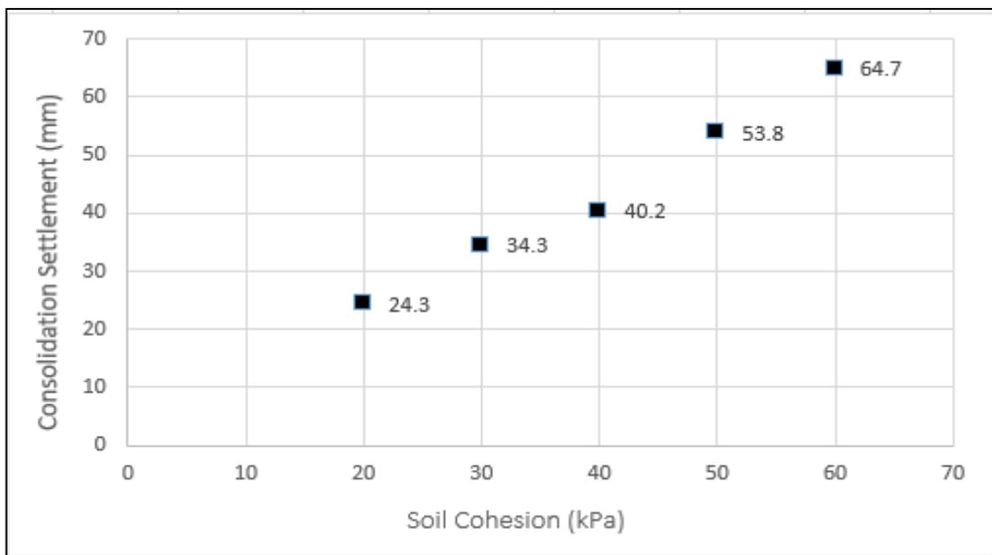
Figure 4.36. The relationship between consolidation settlement for the mid pile tip point of the group bored piles and soil cohesion in the clayey soil under the PLAXIS simulation.
