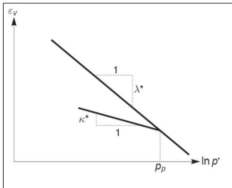
Figure 2.12. Volumetric stress-strain relationship in soft soil model (Naveen and Sitharam, 2011).
