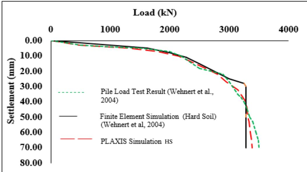
Figure 4.4. Load-settlement behaviour of single bored pile in clayey soil using HS model for Very Fine mesh PLAXIS simulation in comparison to the measured and simulated ones from Wehnert & Vermeer (2004).
