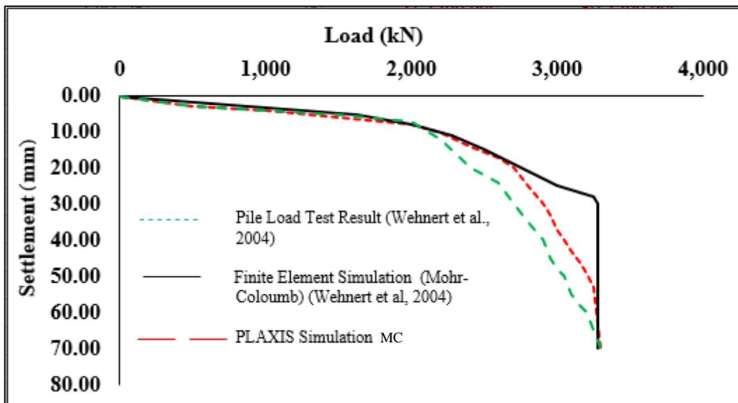
Figure 4.3. Load-settlement behaviour of single bored pile in clayey soil using MC model for Fine mesh PLAXIS simulation in comparison to the measured and simulated ones from Wehnert & Vermeer (2004).
