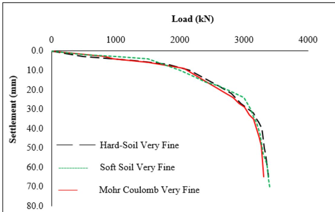
Figure 4.8. Comparison among the load-settlement curves of single bored pile in clayey soil under the PLAXIS simulation for MC, HS and SS models of Very Fine mesh.
