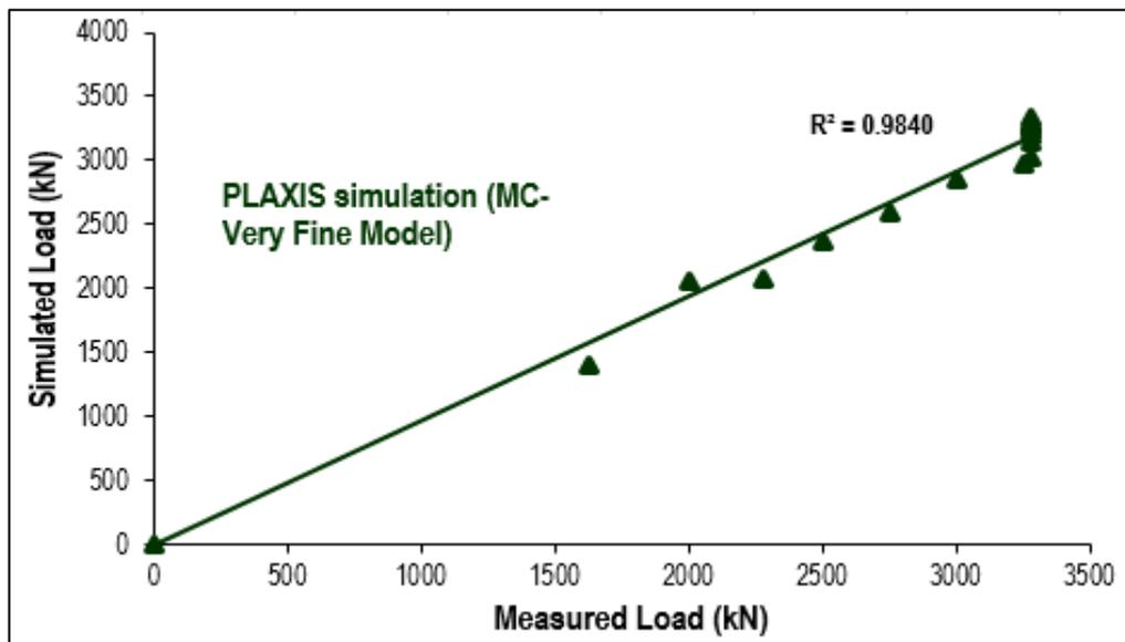
Figure 4.10. The result of  $R^2$  for the simulated load versus measured load for the single bored pile in clayey soil using Mohr-Coulomb model in Very Fine mesh by the PLAXIS simulation.
