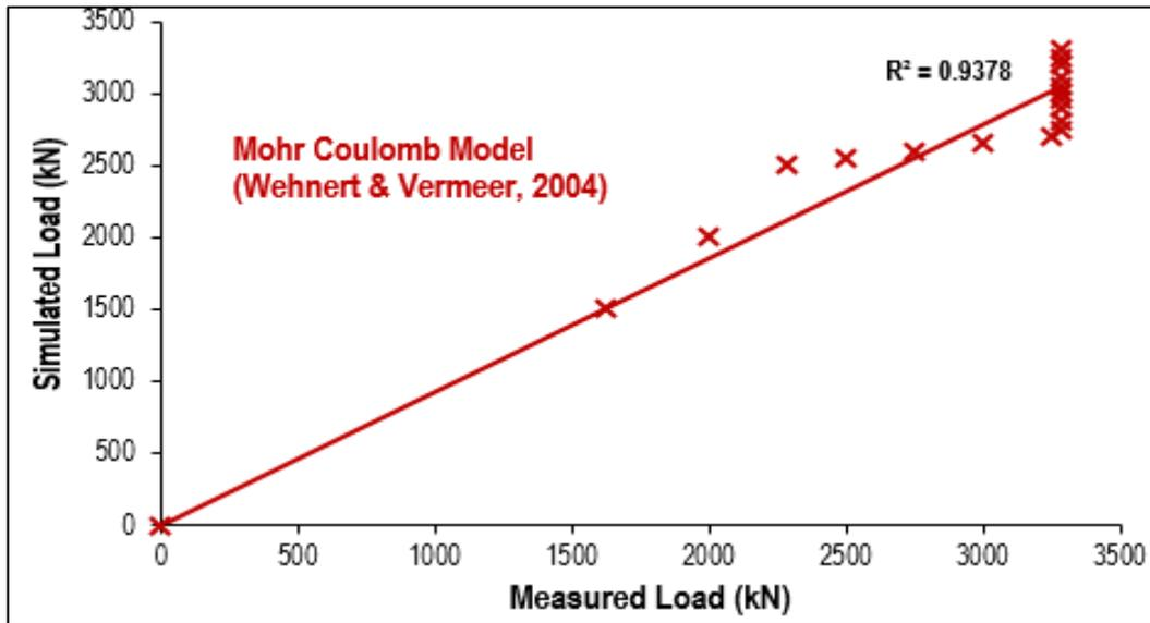
Figure 4.9. The result of  $R^2$  for the simulated load versus measured load for the single bored pile in clayey soil using Mohr-Coulomb model in Very Fine mesh by Wehnert and Vermeer (2004).
