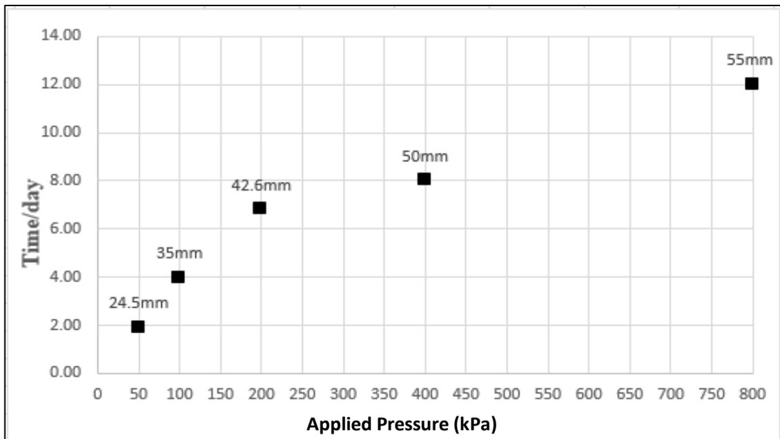
Figure 4.18. The relationship between time and applied pressure for the mid pile tip point of the group bored piles in the clayey soil under the PLAXIS simulation.
