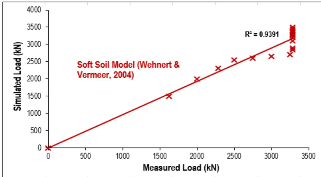
Figure 4.13. The result of  $R^2$  for the simulated load versus measured load for the single bored pile in clayey soil using Soft Soil model in Very Fine mesh by Wehnert and Vermeer (2004).
