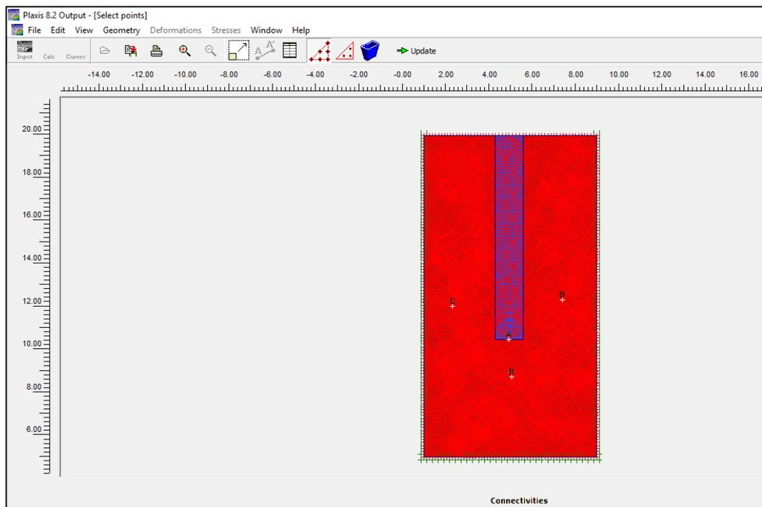
Figure 4.1. Selected tip point of the single bored pile in clayey soil under the PLAXIS simulation.
