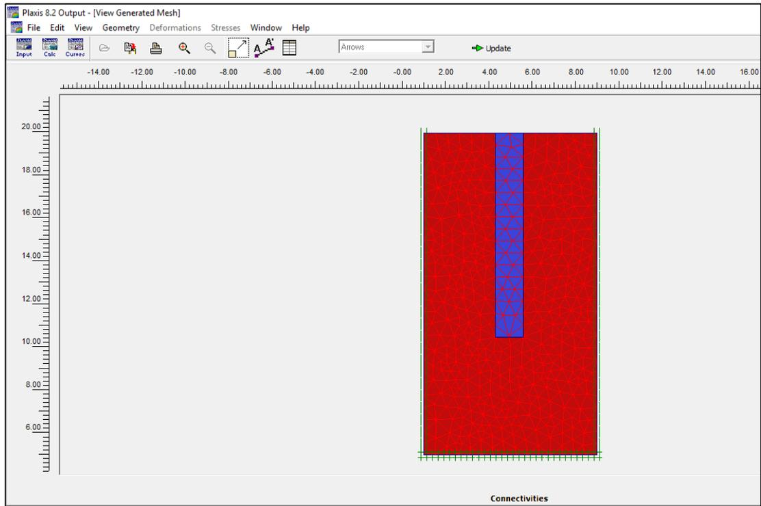
Figure 3.5. Simulation of the single bored pile in clayey soil with very fine mesh.
