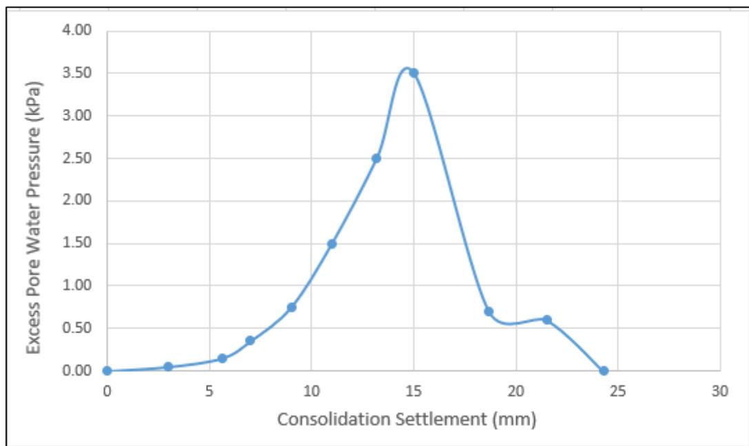
Figure 4.34. The relationship between excess pore water pressure and consolidation settlement for the mid pile tip point of the group bored piles subjected to 50 kPa applied pressure, pile diameter of 1.3 m, pile spacing of 3D, pile slope ratio of 1:2 and soil cohesion of 20 kPa in the clayey soil under the PLAXIS simulation.
