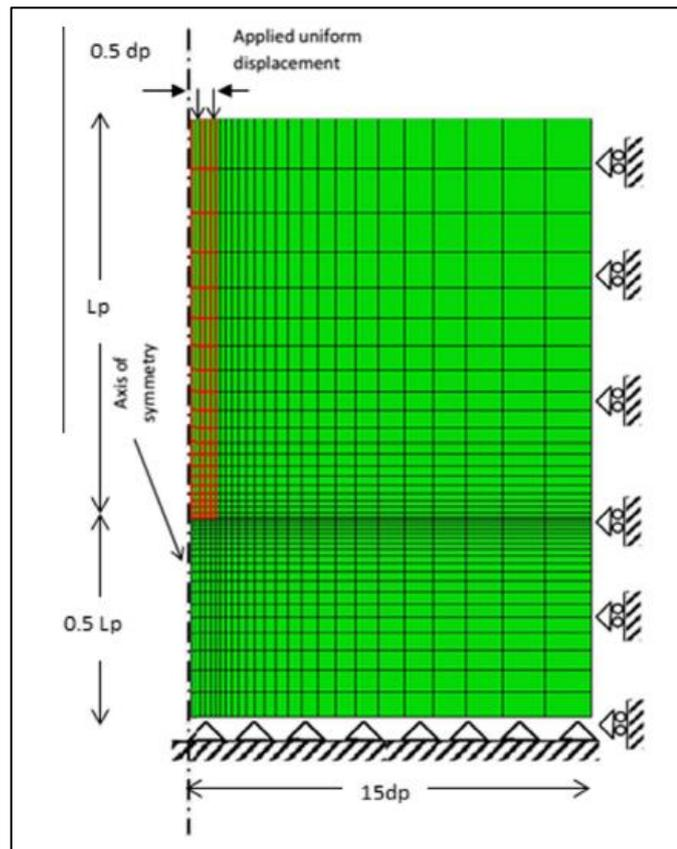
Figure 2.7. Finite element mesh and boundary conditions in full pile simulation (Kamal, 2016).
