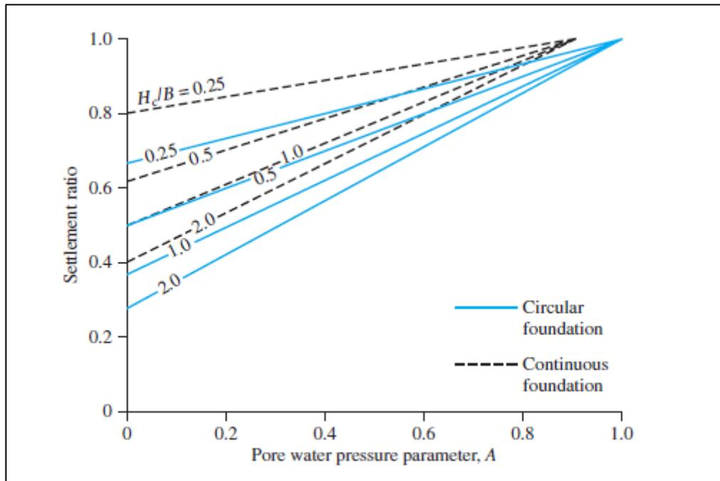
Figure 2.13. Settlement ratios for circular ( $K_{cir}$ ) and continuous ( $K_{str}$ ) foundations (Skempton–Bjerrum modification, 1957).
