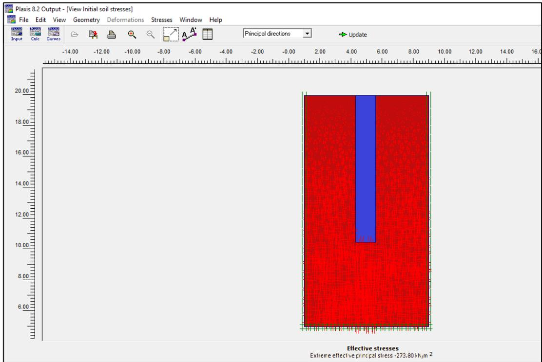
Figure 3.7. Simulation of effective stress distribution of the single bored pile in clayey soil.
