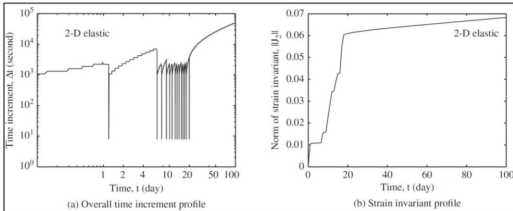
Figure 2.17. Time increments and observed strain history for two-dimensional elastic consolidation (Karim & Oka, 2010).
