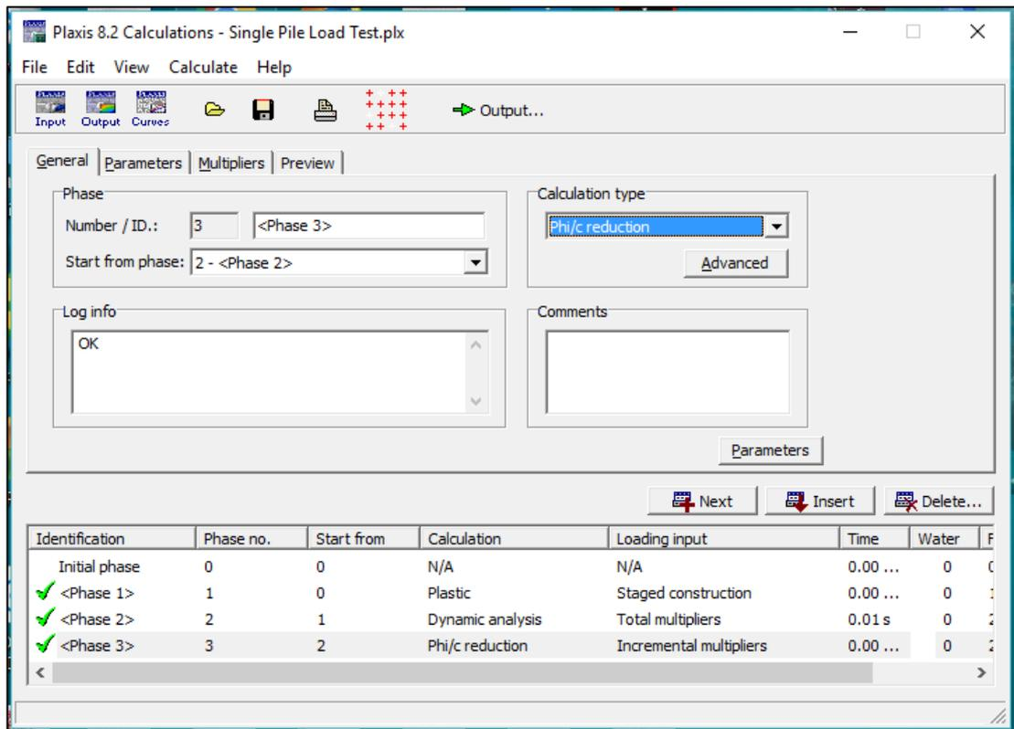
Figure 3.8. The 3 phases of loading input in the software setting for the simulation.
