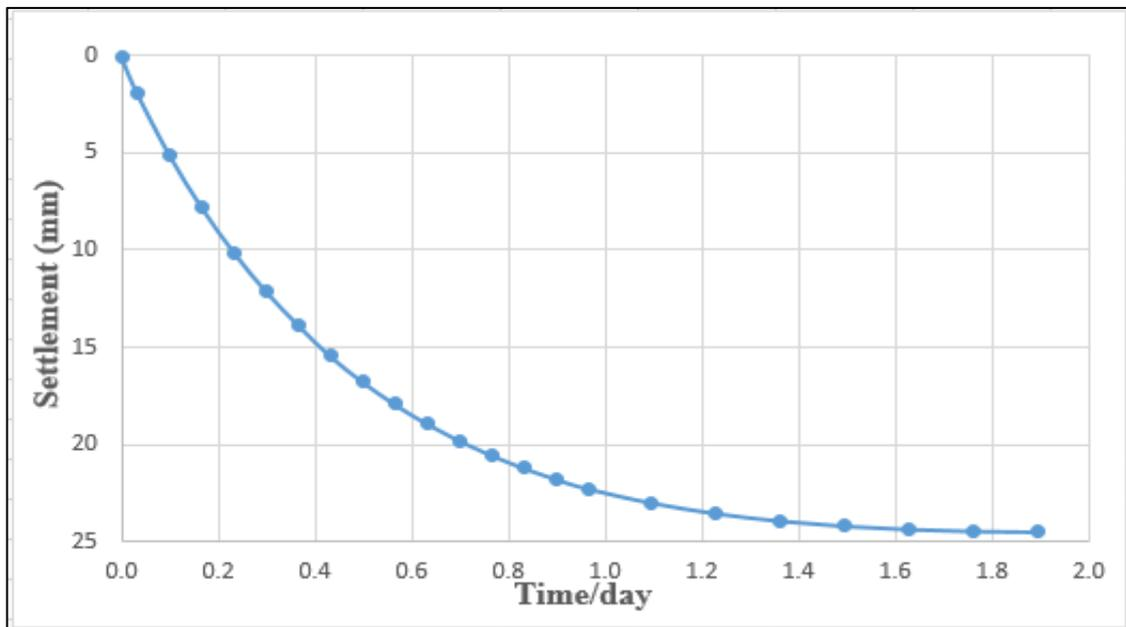
Figure 4.16. The relationship between settlement and time for the mid pile tip point of the group bored piles subjected to 50 kPa applied pressure in the clayey soil under the PLAXIS simulation.
