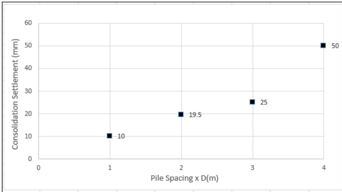
Figure 4.25. The relationship between consolidation settlement for the mid pile tip point of the group bored piles and pile spacing in the clayey soil under the PLAXIS simulation.
