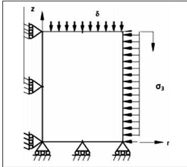
Figure 2.6. Single element used for simulation of single bored pile in ABAQUS software simulation (Kamal, 2016).
