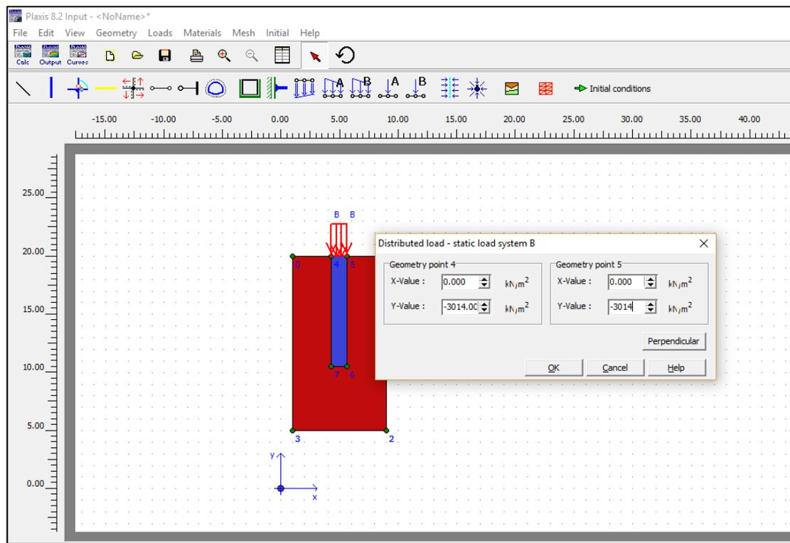
Figure 3.4. The single bored pile simulation in clayey soil under constant load test.
