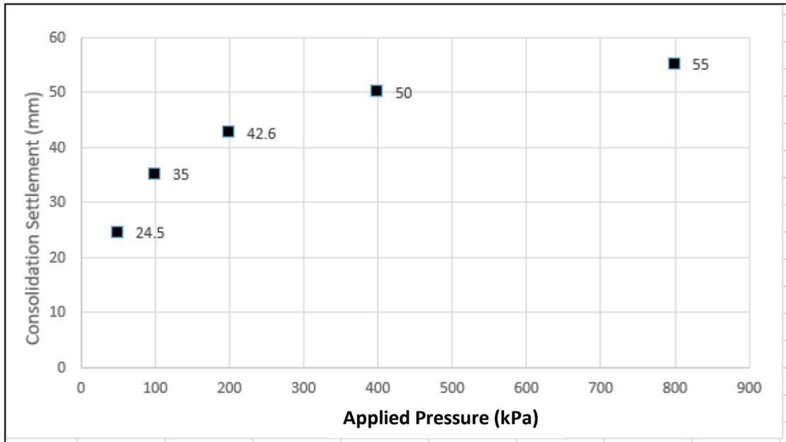
Figure 4.17. The relationship between consolidation settlement and applied pressure for the mid pile tip point of the group bored piles after the dissipation of excess pore water pressure in the clayey soil under the PLAXIS simulation.
