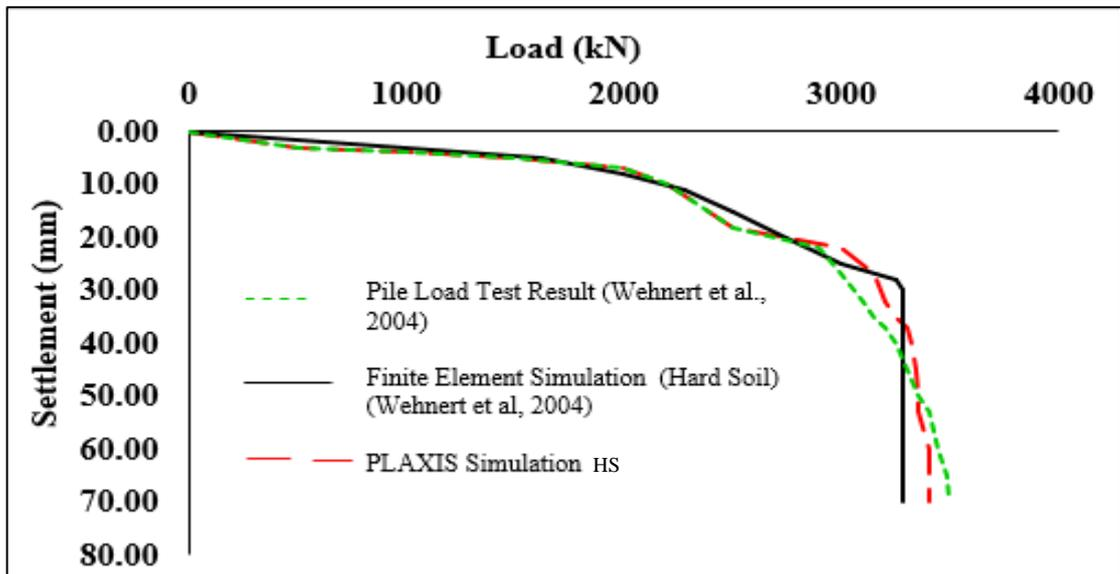
Figure 4.5. Load-settlement behaviour of single bored pile in clayey soil using HS model for Fine mesh PLAXIS simulation in comparison to the measured and simulated ones from Wehnert & Vermeer (2004).
