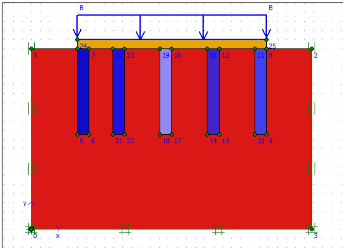
Figure 3.12. Side view of the foundation designed in 5 × 3 group bored pile (Note:  $B$  = Breadth = 9.1 m;  $L$  = Length = 20.8 m, Thickness = 1 m).
