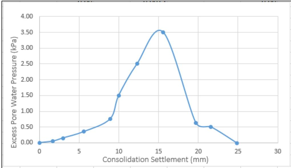
Figure 4.29. The relationship between excess pore water pressure and consolidation settlement for the mid pile tip point of the group bored piles subjected to 50 kPa applied pressure, pile diameter of 1.3 m, pile spacing of 3D and pile slope ratio of 1:2 in the clayey soil under the PLAXIS simulation.
