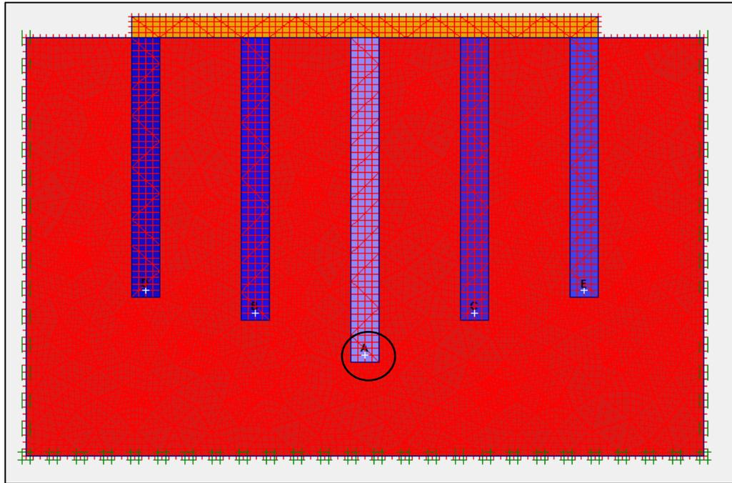
Figure 4.33. Proposed optimal numerical design of the group bored piles in the clayey soil with 50 kPa applied pressure, 1.3 m pile diameter, 3D pile spacing and pile slope ratio 1:2.
