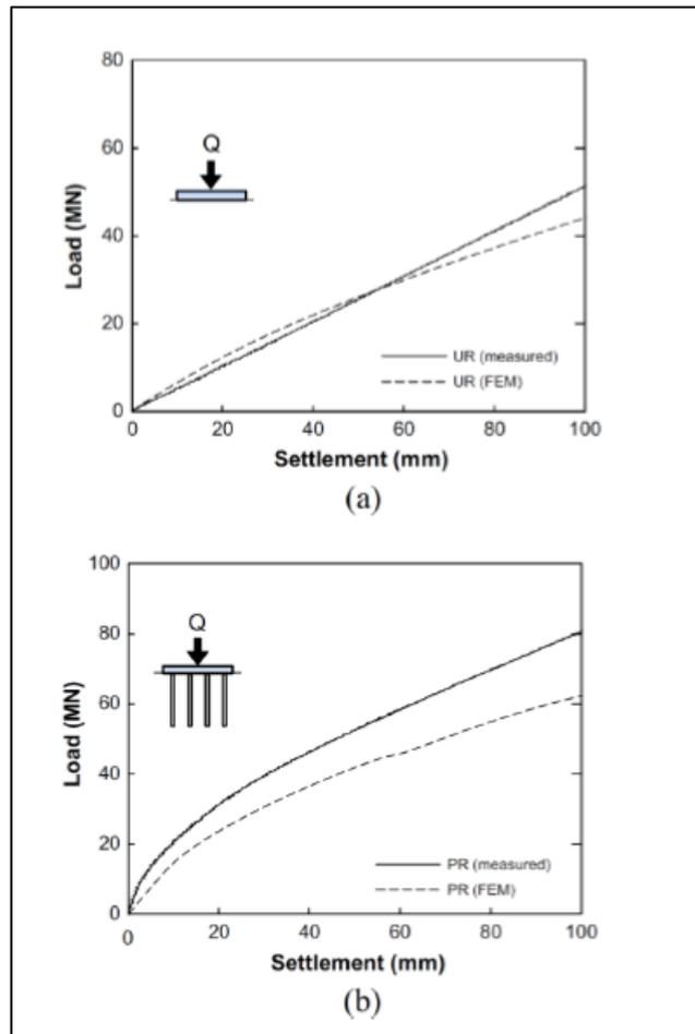
Figure 2.11. Measured and calculated load settlement curve of (a) unpile raft and (b) pile raft (Park and Lee, 2016)
