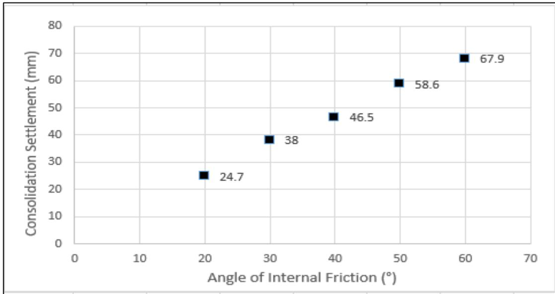
Figure 4.40. The relationship between consolidation settlement for the mid pile tip point of the group bored piles and soil angle of internal friction in the clayey soil under the PLAXIS simulation.
