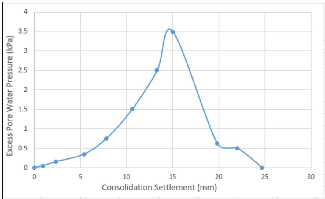
Figure 4.38. The relationship between excess pore water pressure and consolidation settlement for the mid pile tip point of the group bored piles subjected to 50 kPa applied pressure, pile diameter of 1.3 m, pile spacing of 3D, pile slope ratio of 1:2, soil cohesion of 20 kPa and soil angle of internal friction of 20° in the clayey soil under the PLAXIS simulation.
