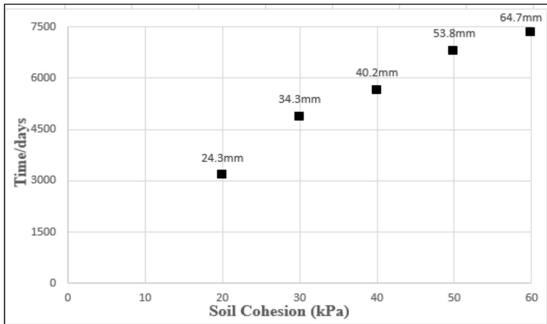
Figure 4.37. The relationship between time and soil cohesion for the mid pile tip point of the group bored piles in the clayey soil under the PLAXIS simulation.
