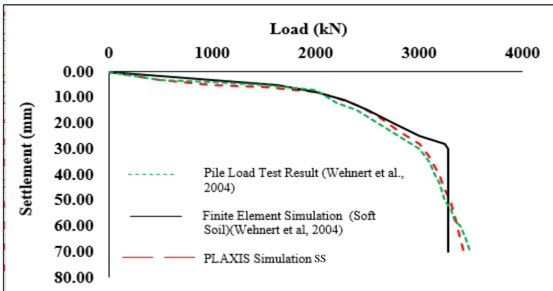
Figure 4.7. Load-settlement behaviour of single bored pile in clayey soil using SS model for Fine mesh PLAXIS simulation in comparison to the measured and simulated ones from Wehnert & Vermeer (2004).
