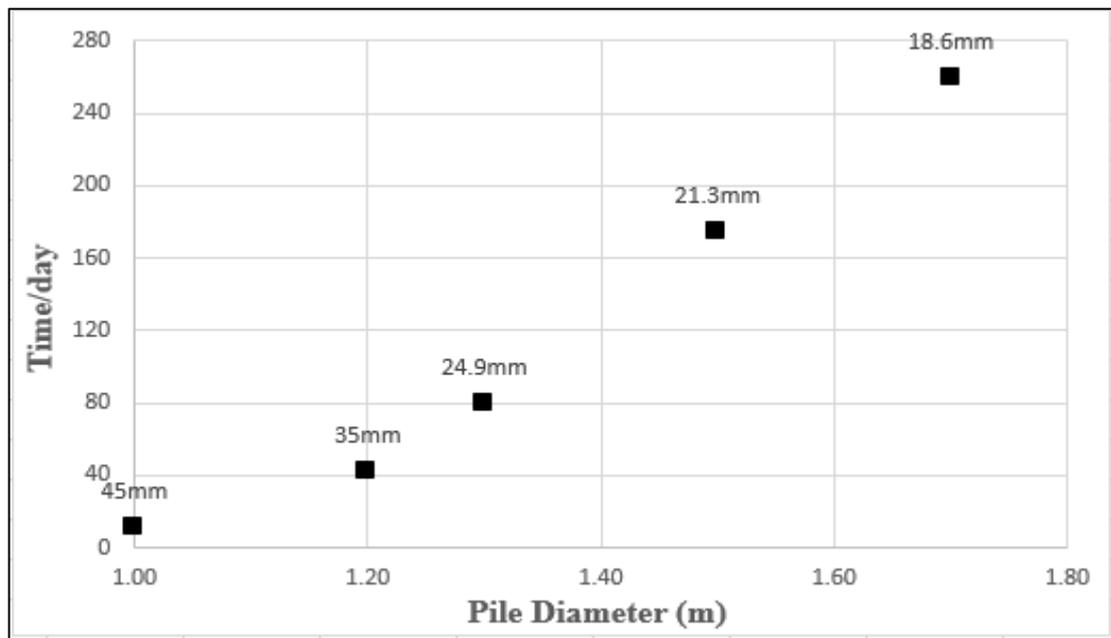
Figure 4.22. The relationship between time and pile diameter for the mid pile tip point of the group bored piles in the clayey soil under the PLAXIS simulation.
