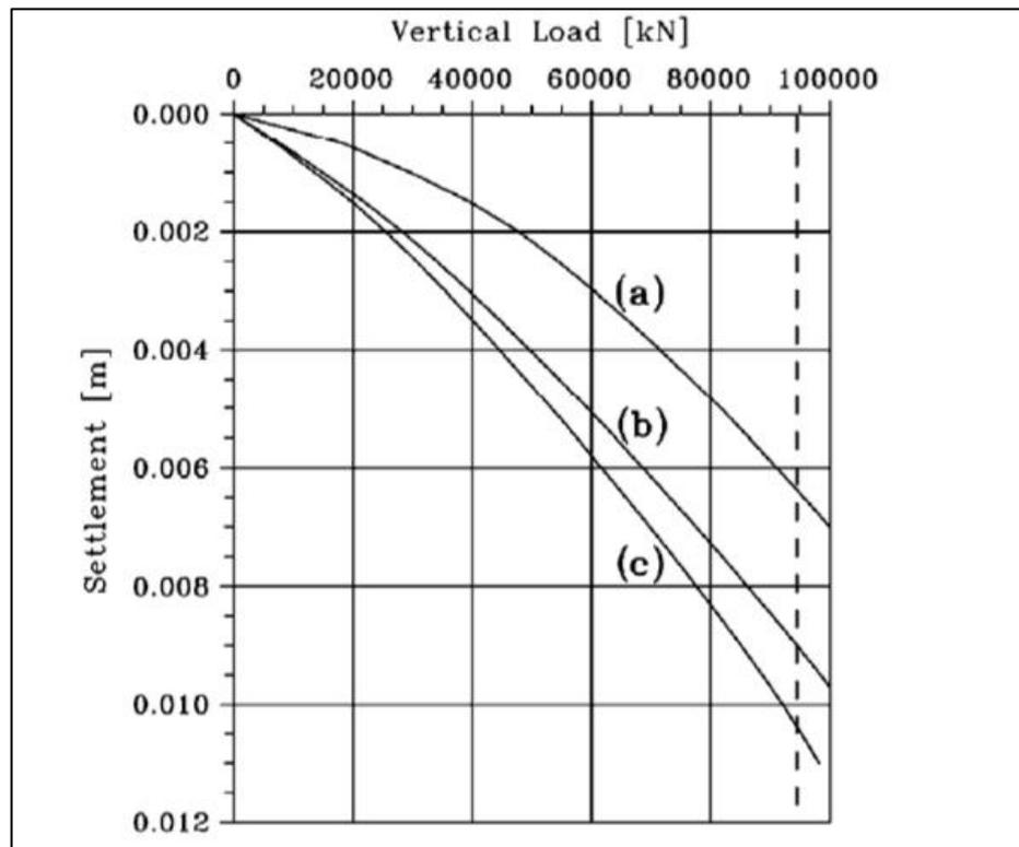
Figure 2.8. Calculated load–settlement curves for the 12 pile group: (a) simple superposition of 12 independent piles; (b) pile group and interaction between soil and foundation mat; and (c) pile group without soil–mat interaction (the dashed line represents the overall working load of the foundation) (Higgins, 2011).
