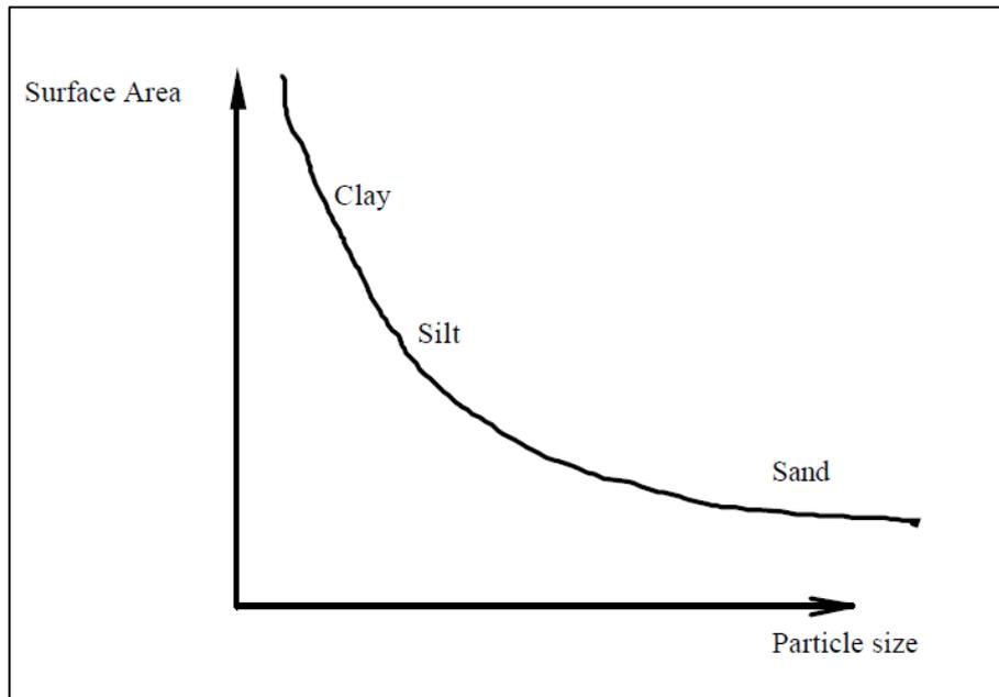
Figure 2.4. Surface area versus particle size of soil (Briaud, 2013).
